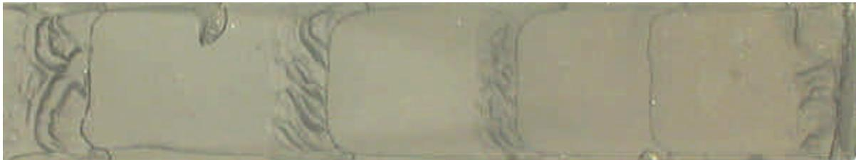
**Figure 6-14** Failure surface of a displacement controlled DCB test. The first four stick-slip crack jumps can be seen. No cavitation is discernable. The magnification is 1x.
