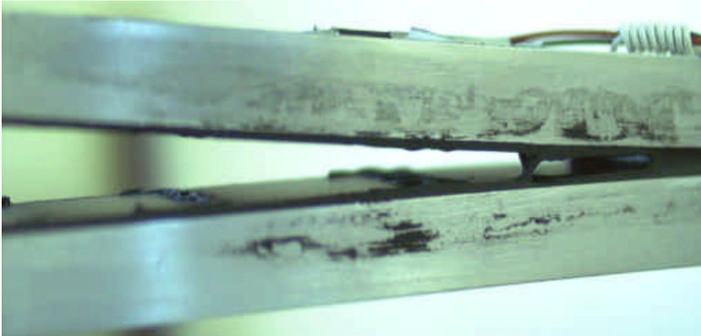
**Figure 6-3** Failure of a displacement controlled DCB sample. The photos show the stick slip behavior as well as the cohesive nature of the failure.
