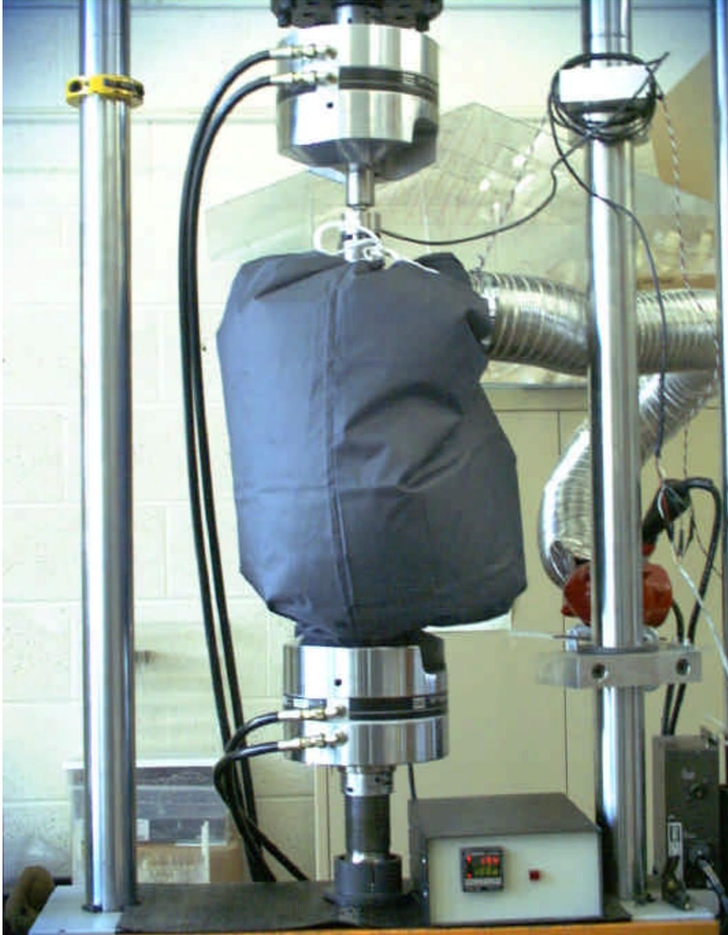
**Figure 5-2** Elevated temperature fatigue testing arrangement.
