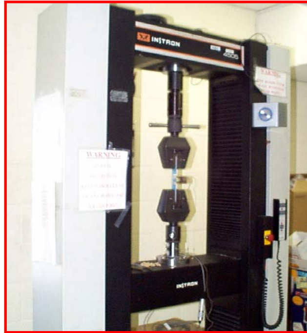
Figure 4.2 Typical tension test setup
