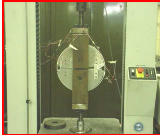
b) 12-inch split disk fixture
