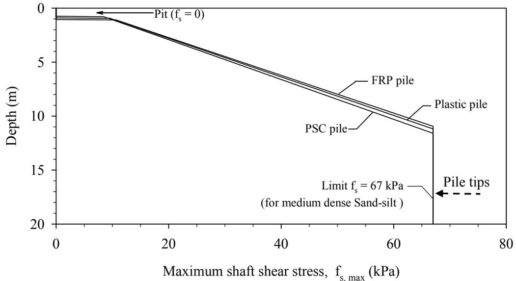
**Figure 7.12 Maximum shear stress distribution along pile shaft, according to API (1993)**
