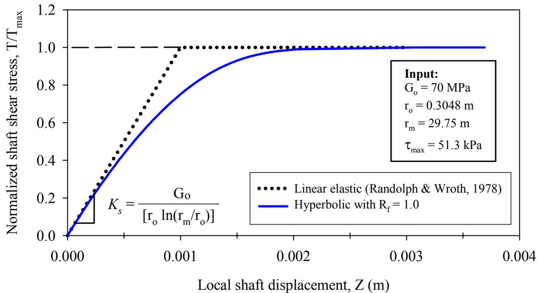
**Figure 7.25 Hyperbolic T-Z Curve based on Randolph and Wroth (1978)**
