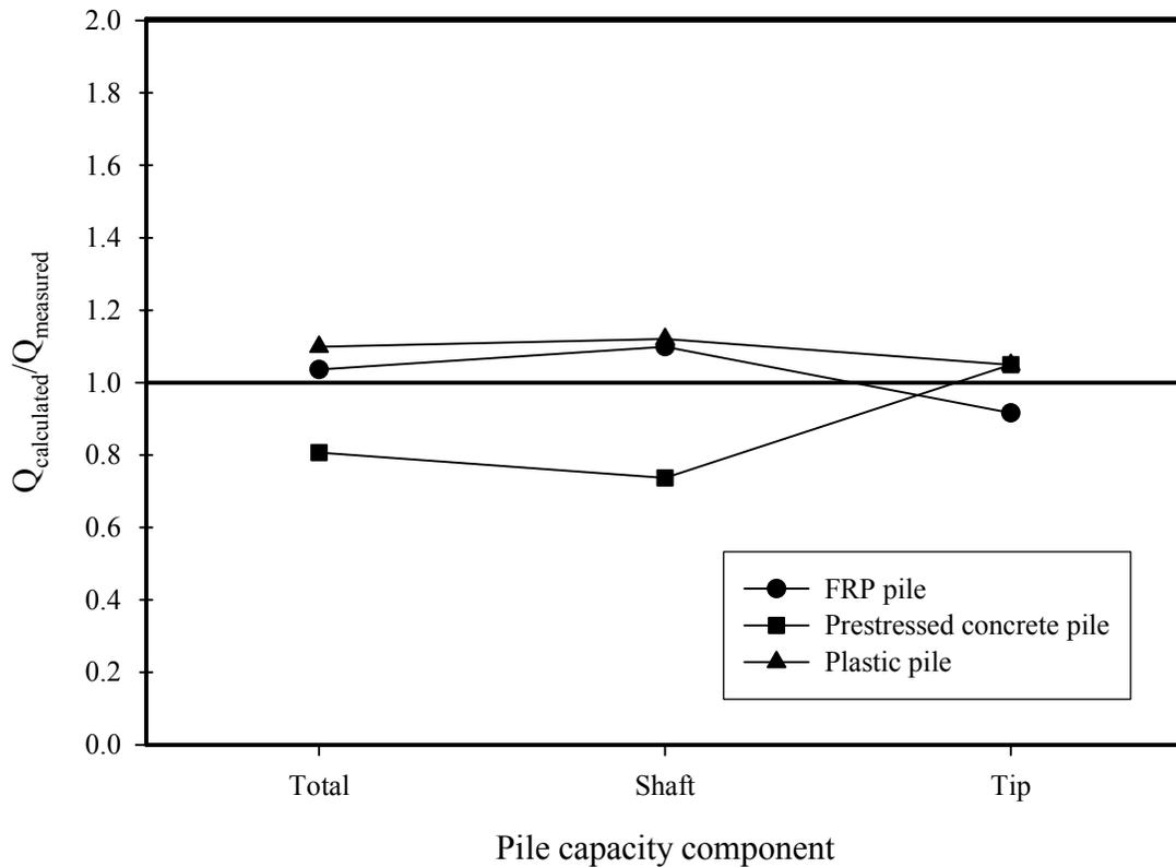
**Figure 7.9 Accuracy of IC method predictions using  $\delta$  values from interface shear tests**
