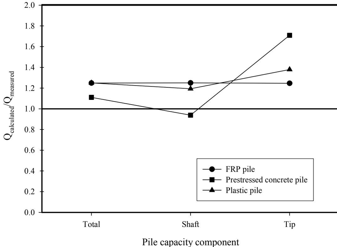
**Figure 7.8 Accuracy of LCPC method predictions using “concrete pile” assumption**
