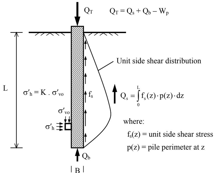
**Figure 7.1. Load Transfer in an Axially Loaded Pile**
