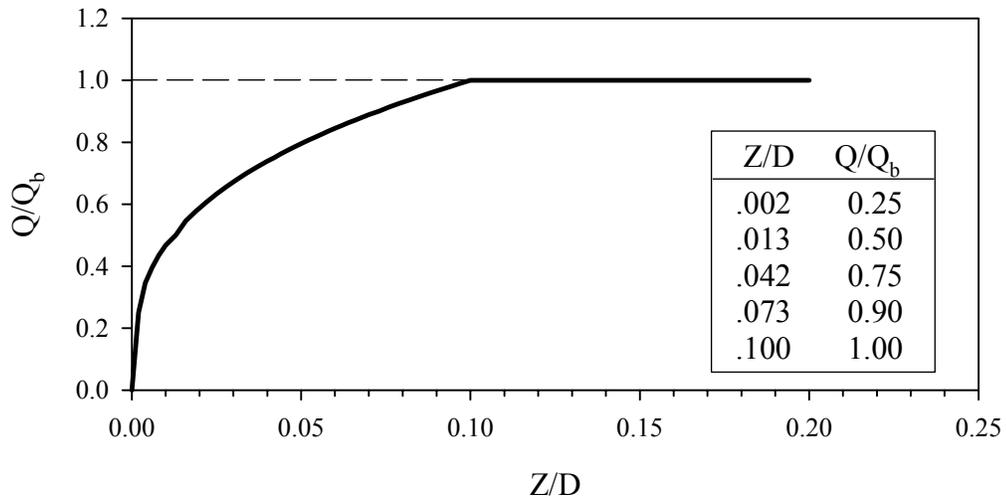
**Figure 7.11 Pile Tip Load – Pile Tip Displacement Curve (Q-Z) (API 1993)**
