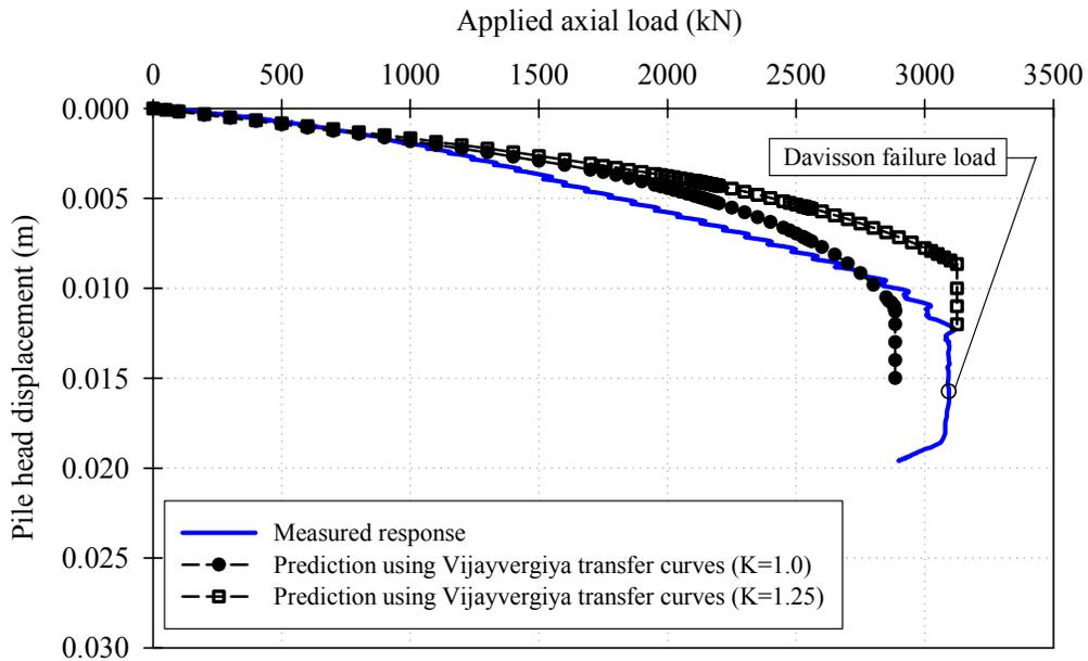
**Figure 7.19 Settlement predictions, for the concrete pile, using Vijayvergiya (1977)**
