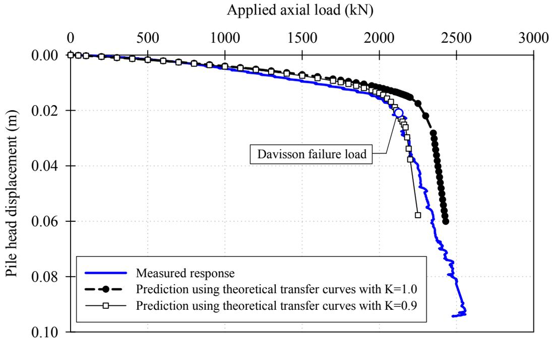
**Figure 7.32 Settlement predictions for the plastic pile using theoretically derived transfer curves**
