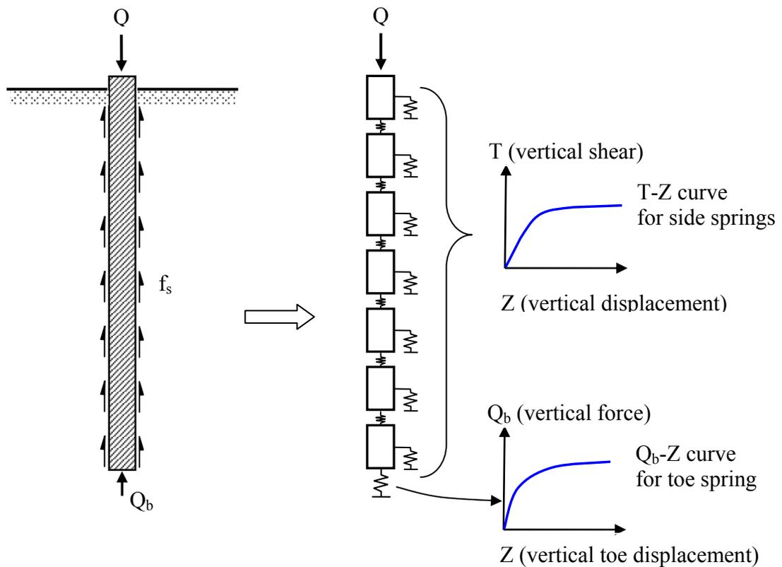
**Figure 7.10 Idealized model used in T-Z load transfer analyses**
