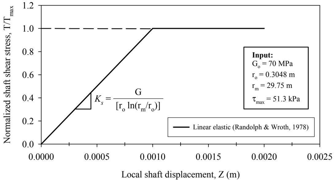
**Figure 7.23 Linear T-Z Curve obtained using Randolph and Wroth (1978)**
