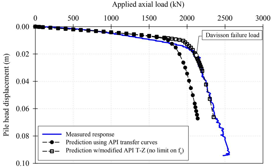
**Figure 7.15 Settlement predictions for the plastic pile using API (1993)**
