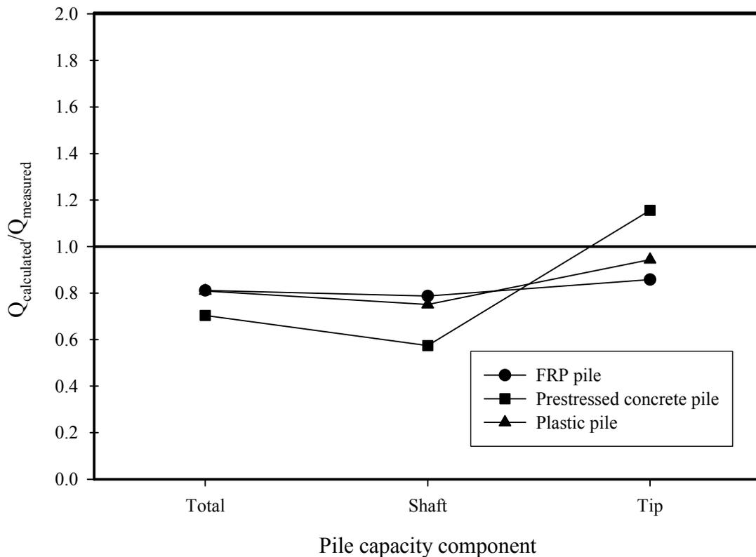
**Figure 7.5 Accuracy of API method predictions using  $\delta$  values from Table 7.1**
