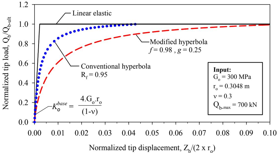
**Figure 7.28 Theoretically derived Q-Z curve using Boussinesq's theory, and the modified hyperbola from Fahey and Carter (1993).**
