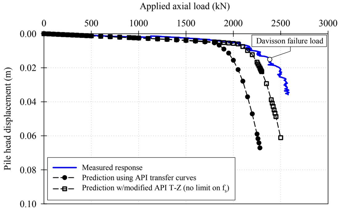
**Figure 7.14 Settlement predictions for the FRP pile using API (1993)**
