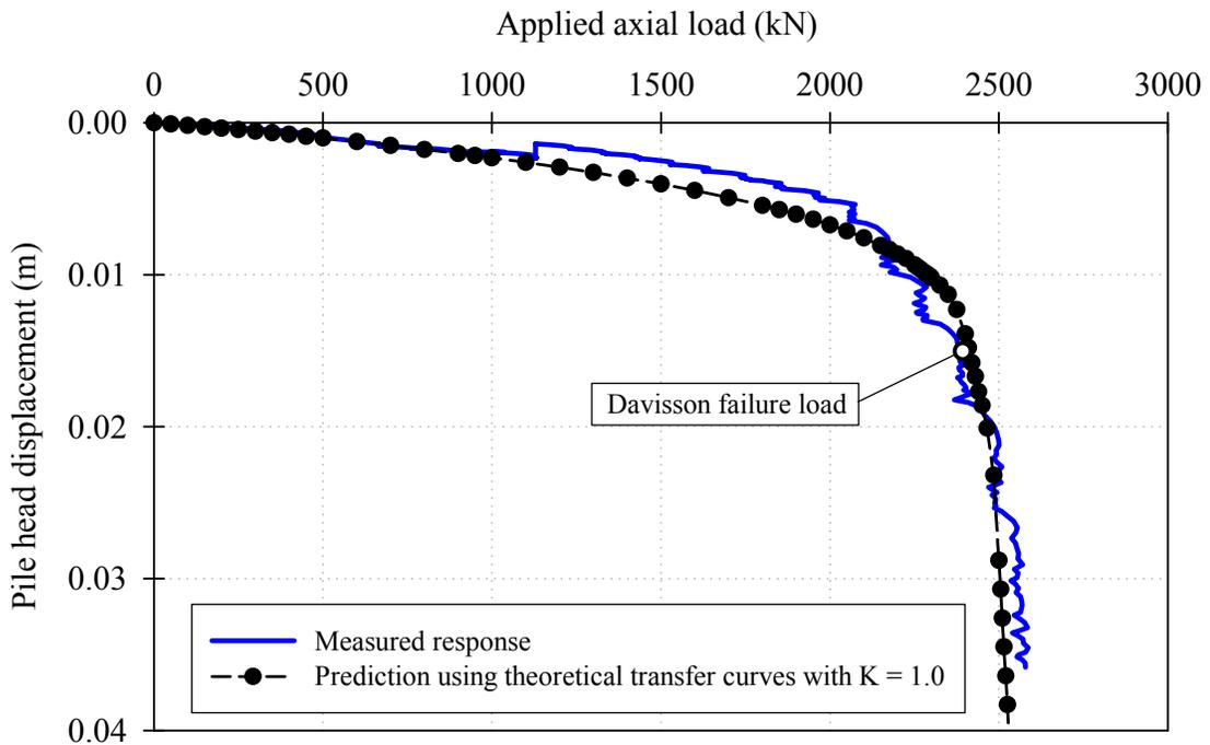
**Figure 7.31 Settlement prediction for the FRP pile using theoretically derived transfer curves**
