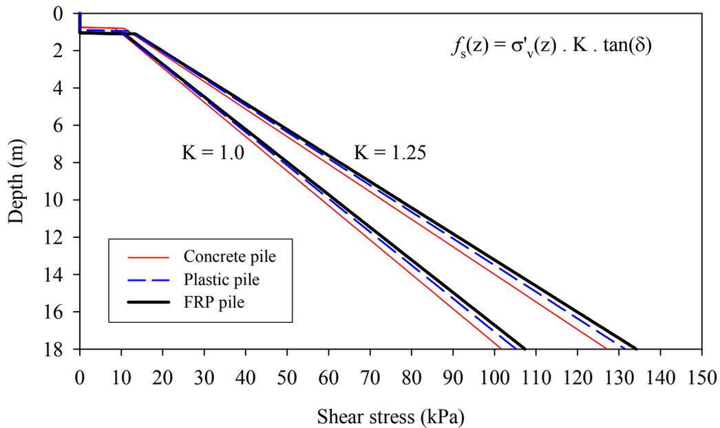
**Figure 7.18 Maximum shear stress distributions used in predictions using Vijayvergiya (1977)**
