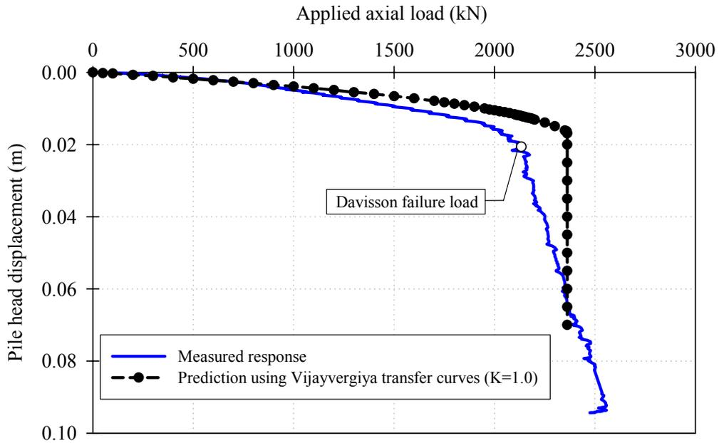
**Figure 7.21 Settlement predictions, for the Plastic pile, using Vijayvergiya (1977)**
