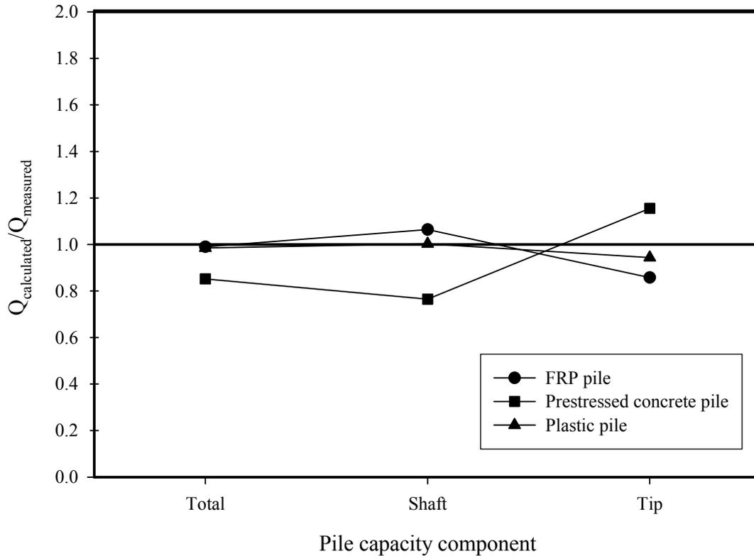
**Figure 7.6 Accuracy of API method predictions using  $\delta$  values from interface shear tests**
