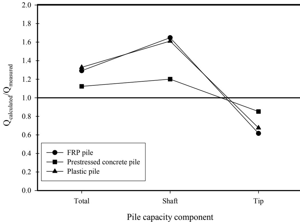
**Figure 7.4 Accuracy of Nordlund method predictions using  $\delta$  values from interface shear tests**
