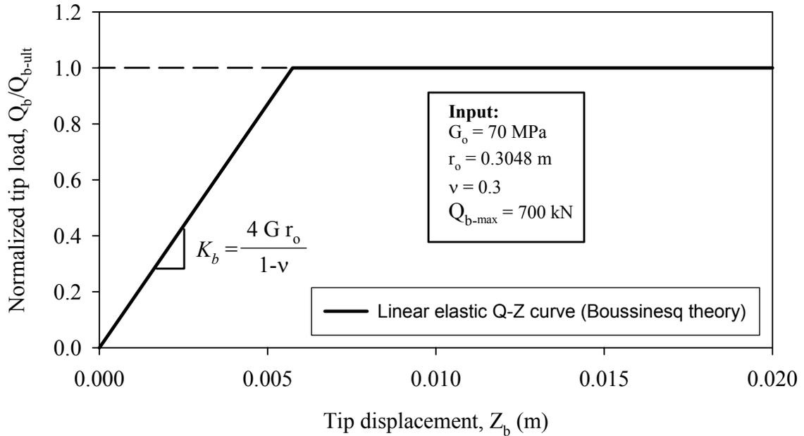
**Figure 7.24 Linear  $Q_b$ - $Z$  curve obtained using Boussinesq's theory**
