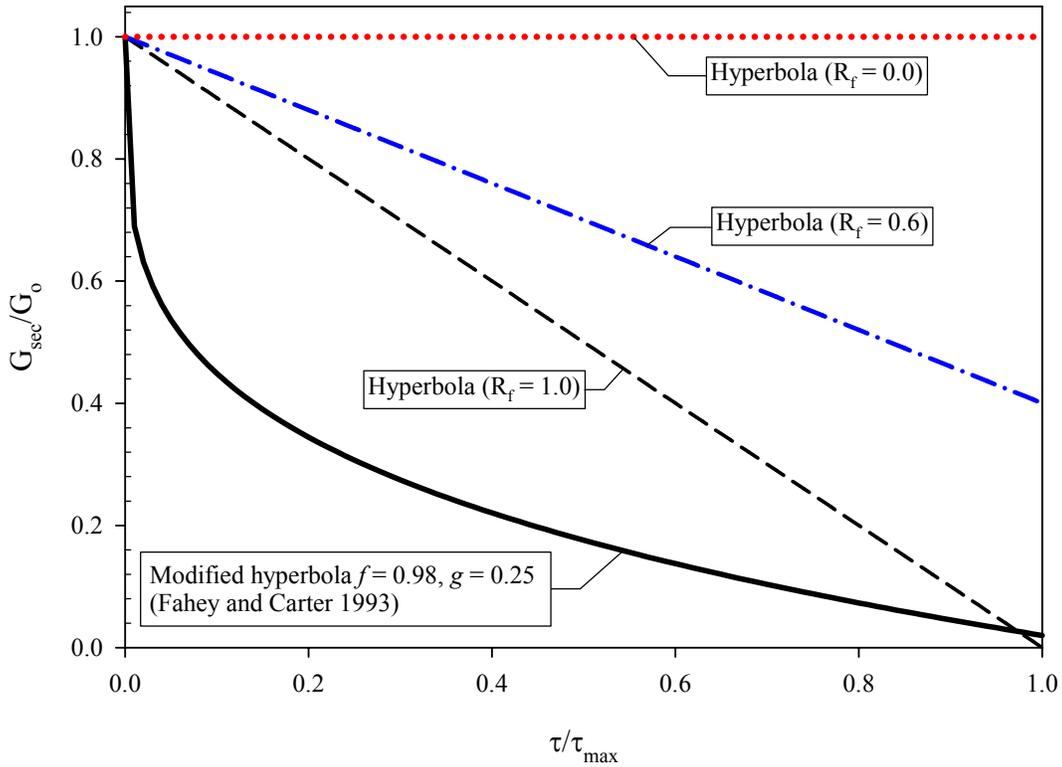
**Figure 7.26 Variation of secant shear modulus for different hyperbolic-type models**
