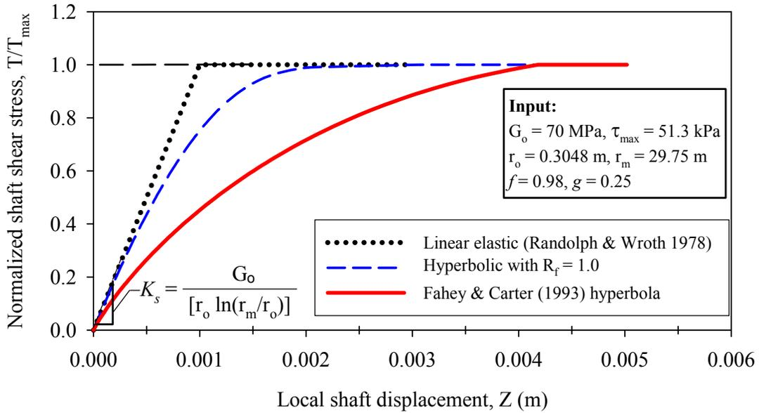
**Figure 7.27 Theoretically derived T-Z curve using concentric cylinders, and the modified hyperbola from Fahey and Carter (1993).**
