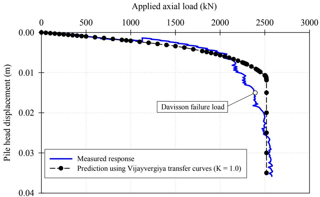
**Figure 7.20 Settlement predictions, for the FRP pile, using Vijayvergiya (1977)**
