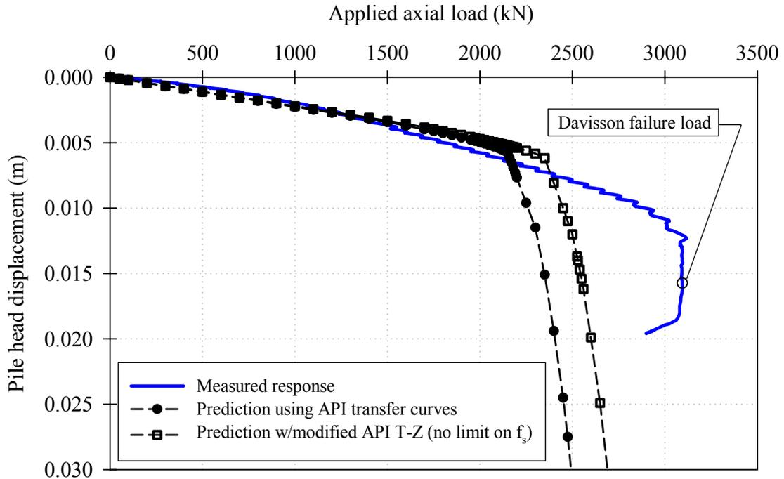
**Figure 7.13 Settlement predictions for the prestressed concrete pile using API (1993)**
