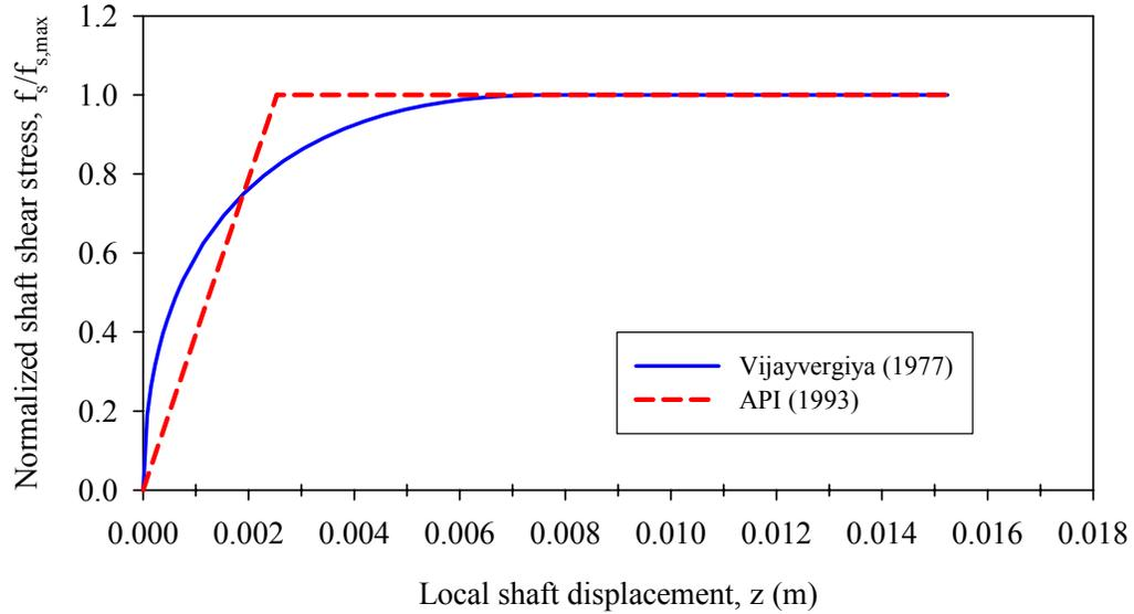
**Figure 7.16 Normalized T-Z curves according to API (1993) and Vijayvergiya (1977)**
