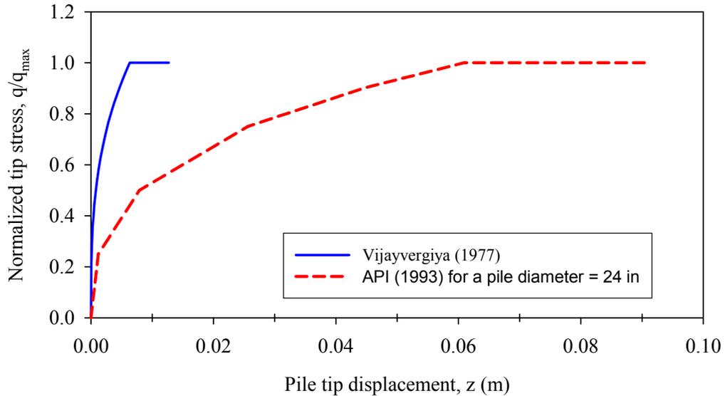
**Figure 7.17 Normalized Q-Z curves according to Vijayvergiya (1977) and API (1993)**
