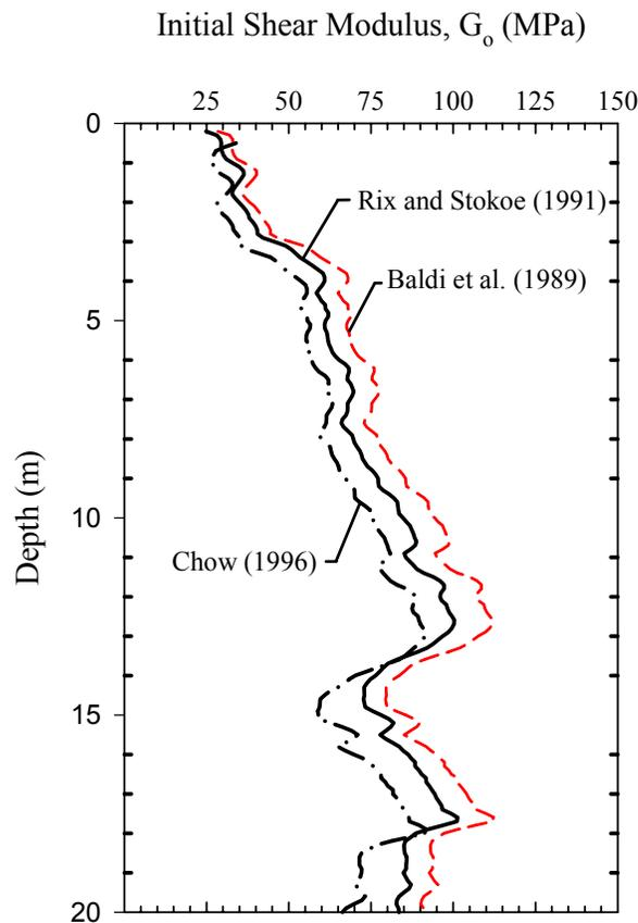
**Figure 7.29 Route 351 Initial Shear Modulus Profile from CPT Correlations**
