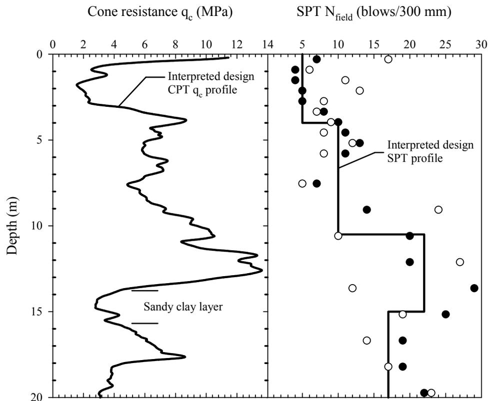
**Figure 7.2 Interpreted Average CPT and SPT Design Profiles for Rte 351 test site**
