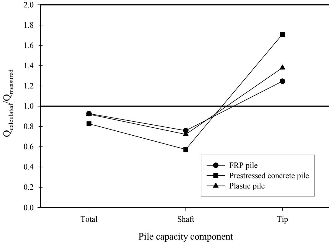
**Figure 7.7 Accuracy of LCPC method predictions using “steel pile” assumption**
