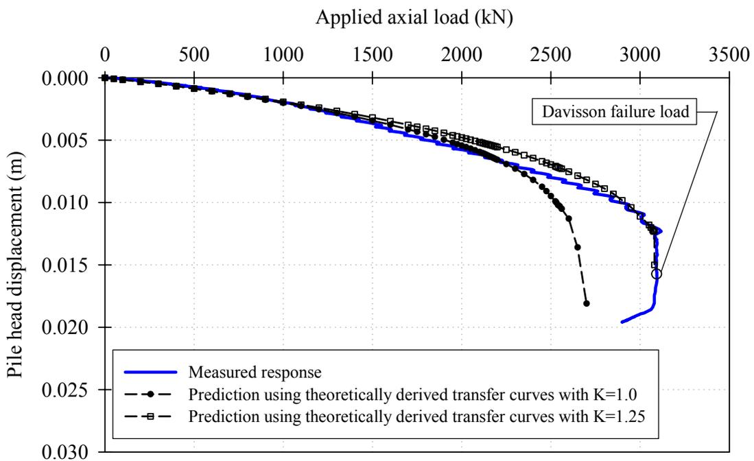
**Figure 7.30 Settlement predictions for the concrete pile using theoretically derived transfer curves**
