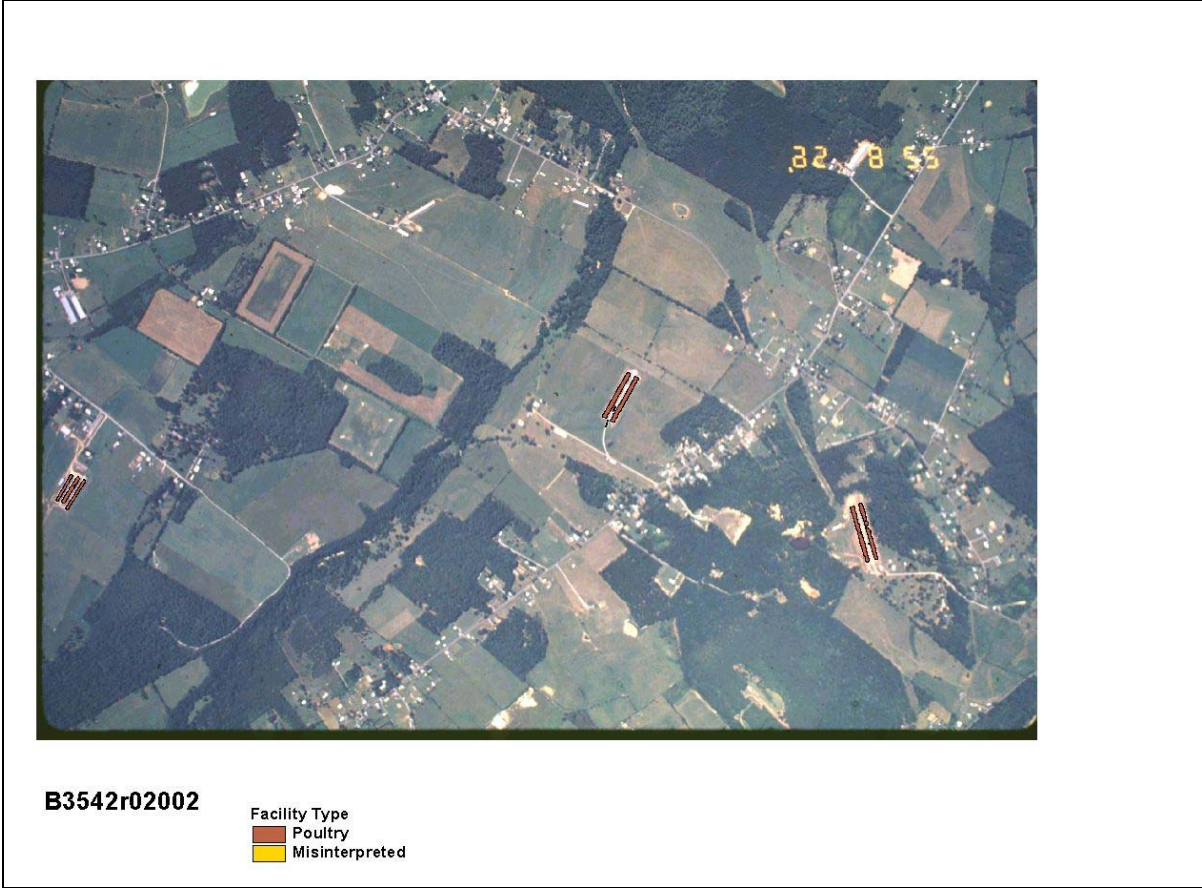
Figure A-20. Automated identification results for slide B3542r02002 (7 poultry houses identified, 0 missed, 0 misinterpreted).
