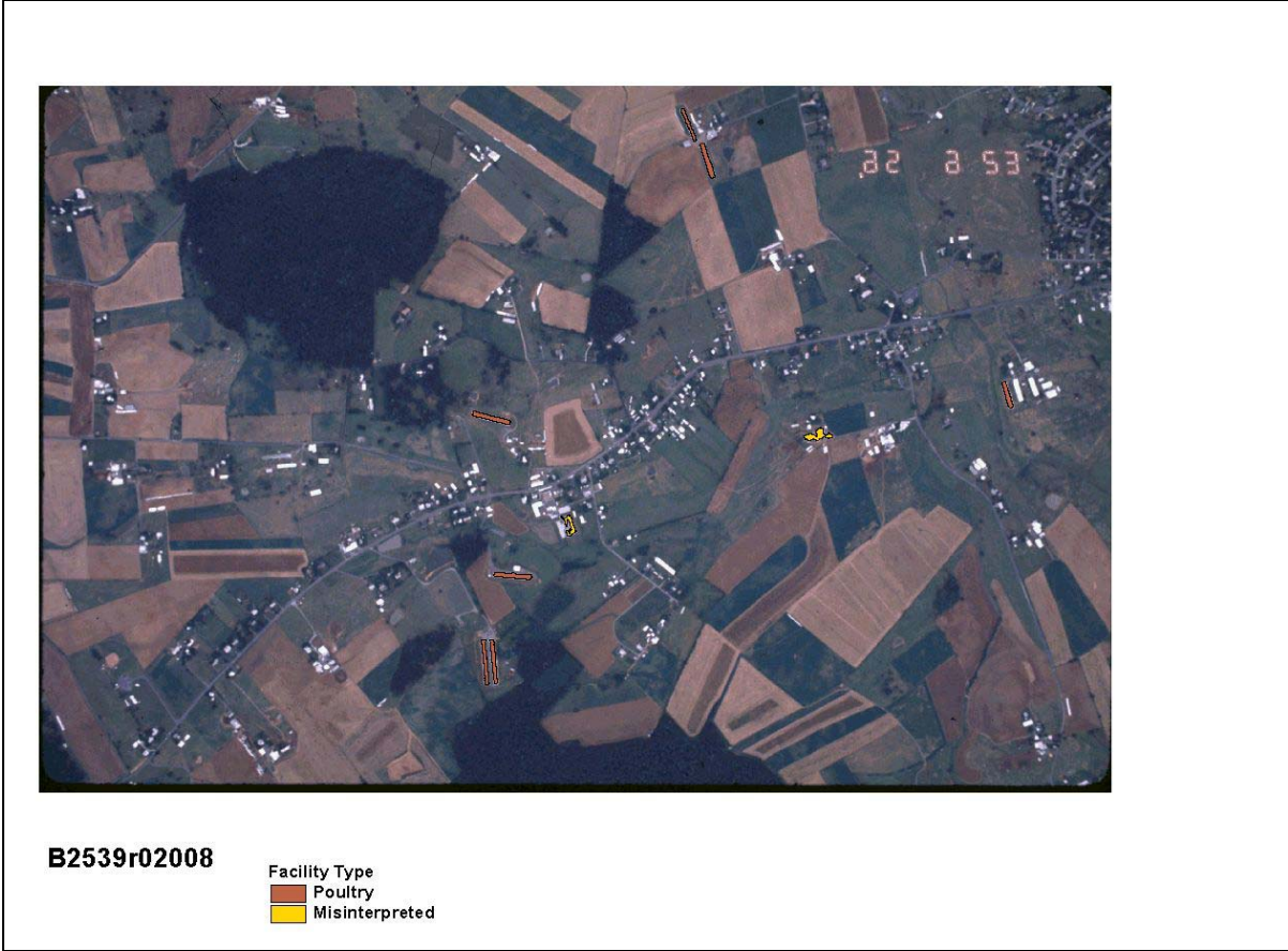
Figure A-14. Automated identification results for slide B2539r02008 (7 poultry houses identified, 0 missed, 2 misinterpreted).
