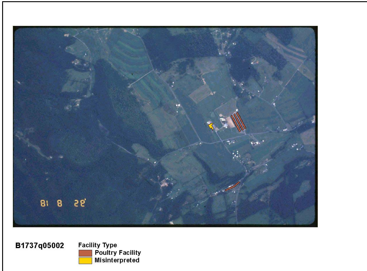
Figure A-1 Automated identification results for slide B1737q05002 (4 poultry houses identified, 0 missed, 1 misinterpreted).
