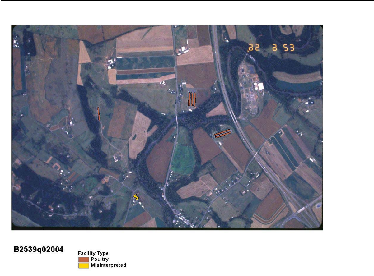
Figure A-10 Automated identification results for slide B2539q02004 (6 poultry houses identified, 0 missed, 1 misinterpreted).
