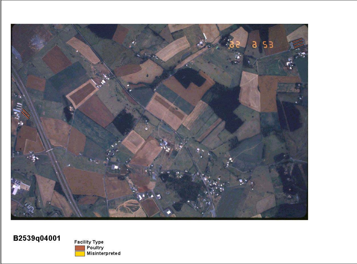
Figure A-11. Automated identification results for slide B1939q04001 (2 poultry houses identified, 0 missed, 0 misinterpreted).
