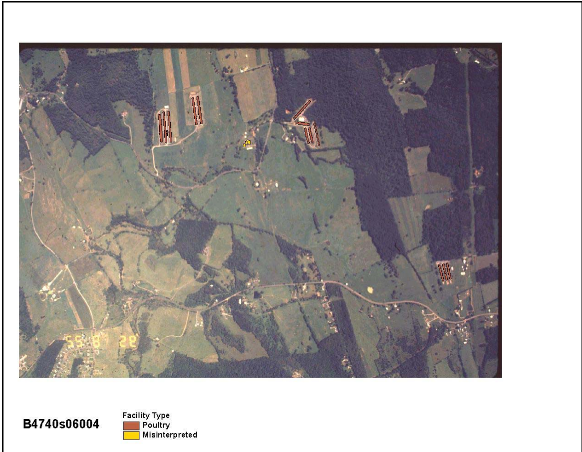
Figure 4-19. Slide image (B4740s06004) with thirteen poultry houses correctly identified and one object (dairy) misidentified.
