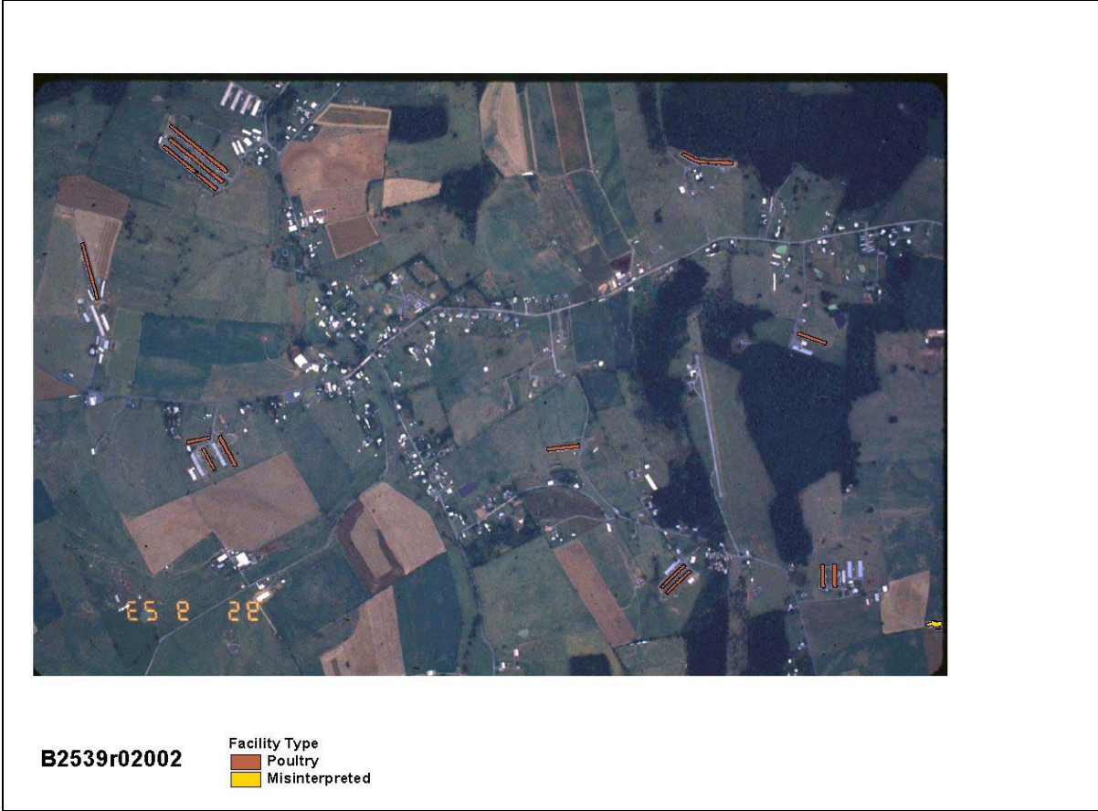
Figure A-13. Automated identification results for slide B2539r02002 (12 poultry houses identified, 0 missed, 1 misinterpreted).
