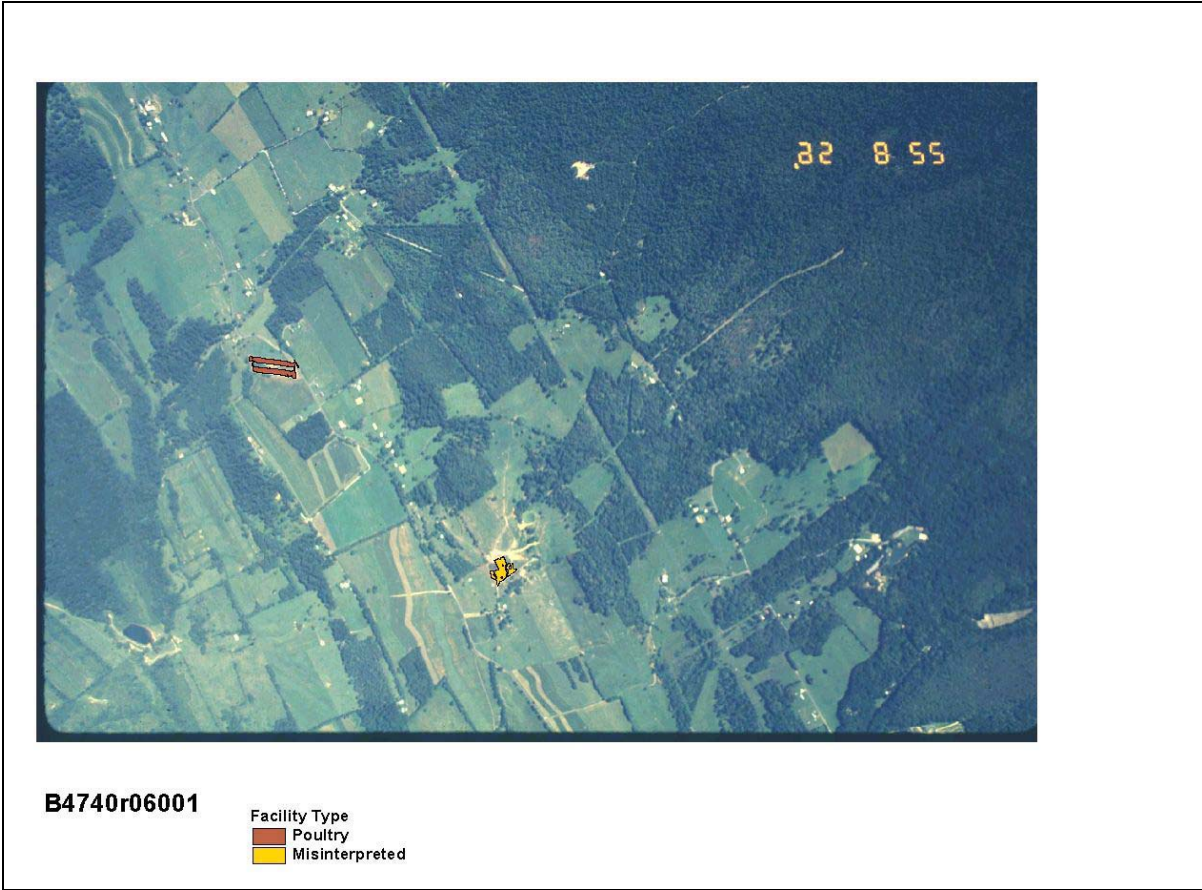
Figure A-23. Automated identification results for slide B4740r06001 (2 poultry houses identified, 0 missed, 1 misinterpreted).
