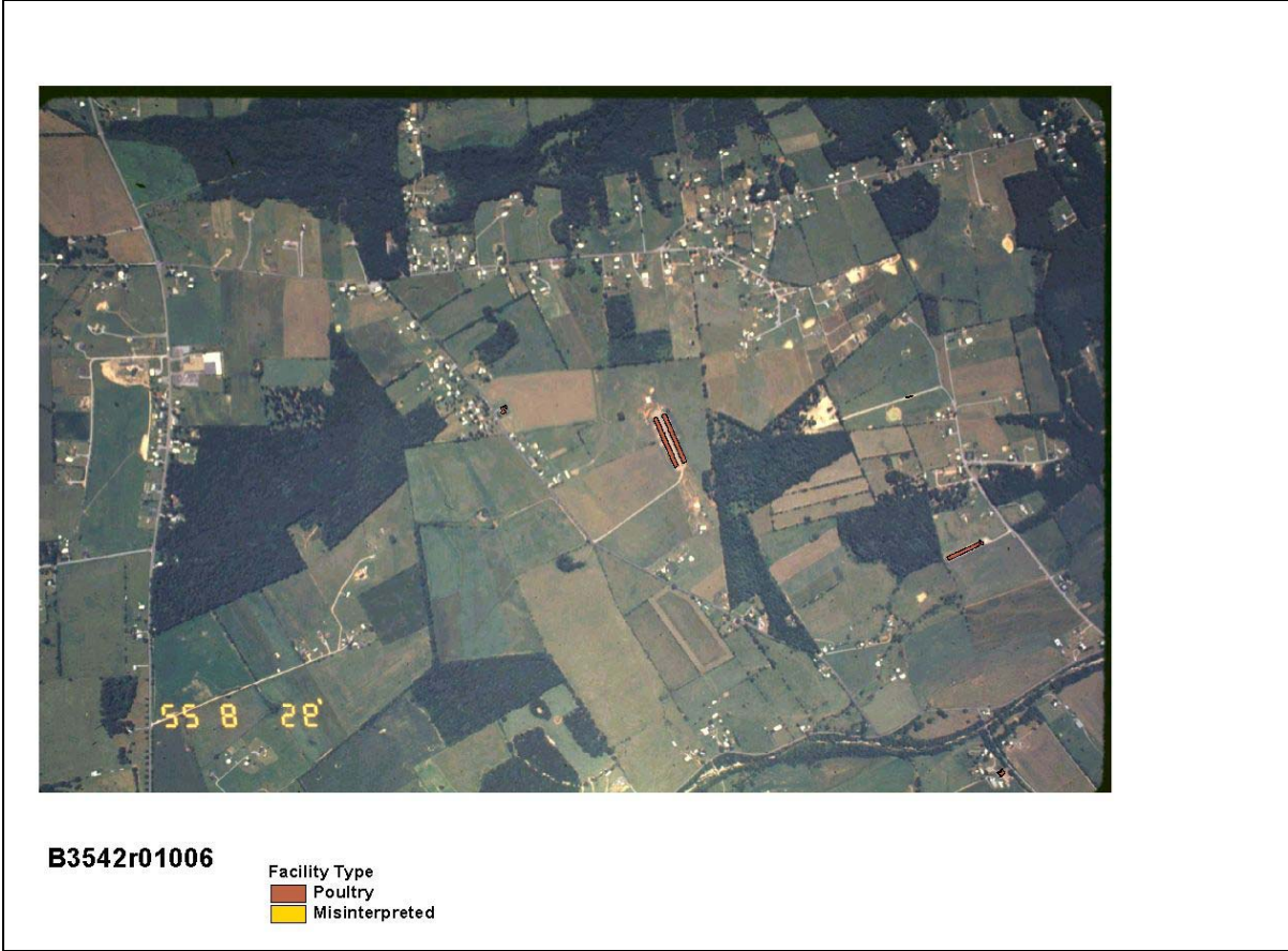
Figure A-19. Automated identification results for slide B3542r01006 (3 poultry houses identified, 0 missed, 0 misinterpreted).
