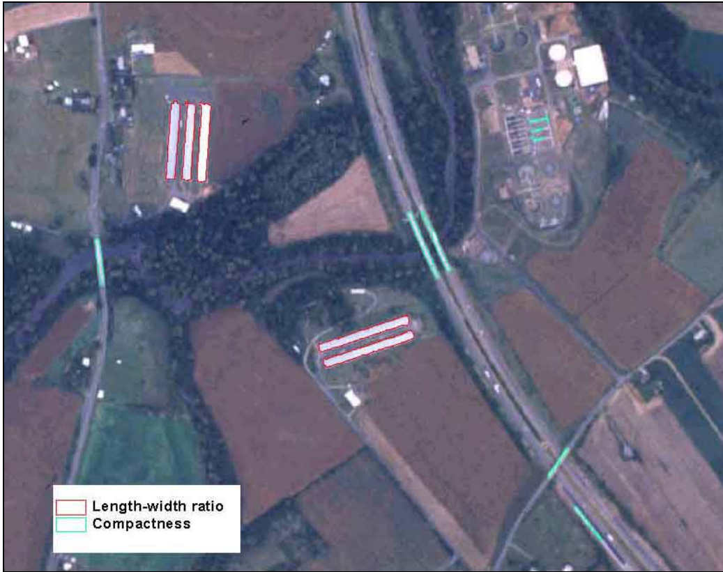
Figure 4-17. An example of polygons selected based on compactness and length-width.
