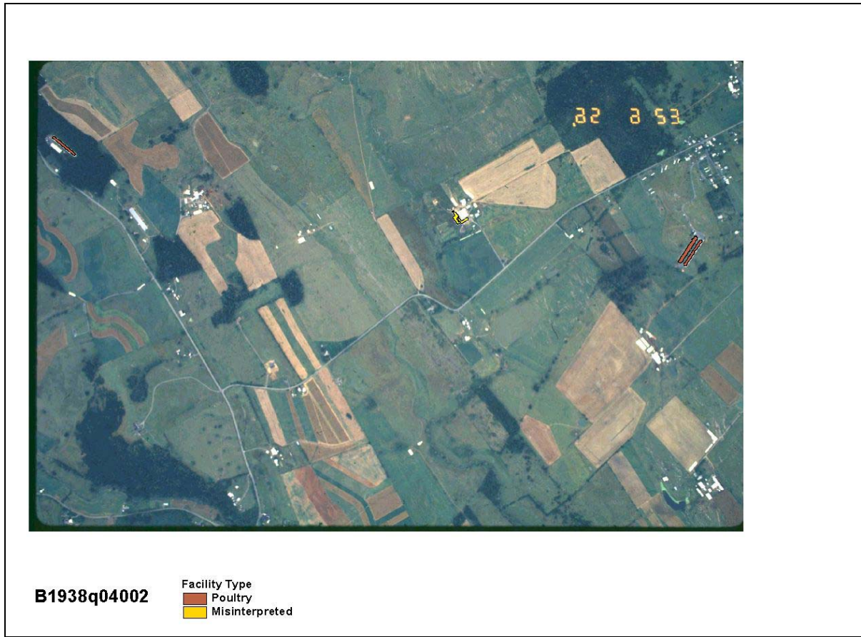
Figure A-5. Automated identification results for slide B1938q04002 (3 poultry houses identified, 0 missed, 1 misinterpreted).
