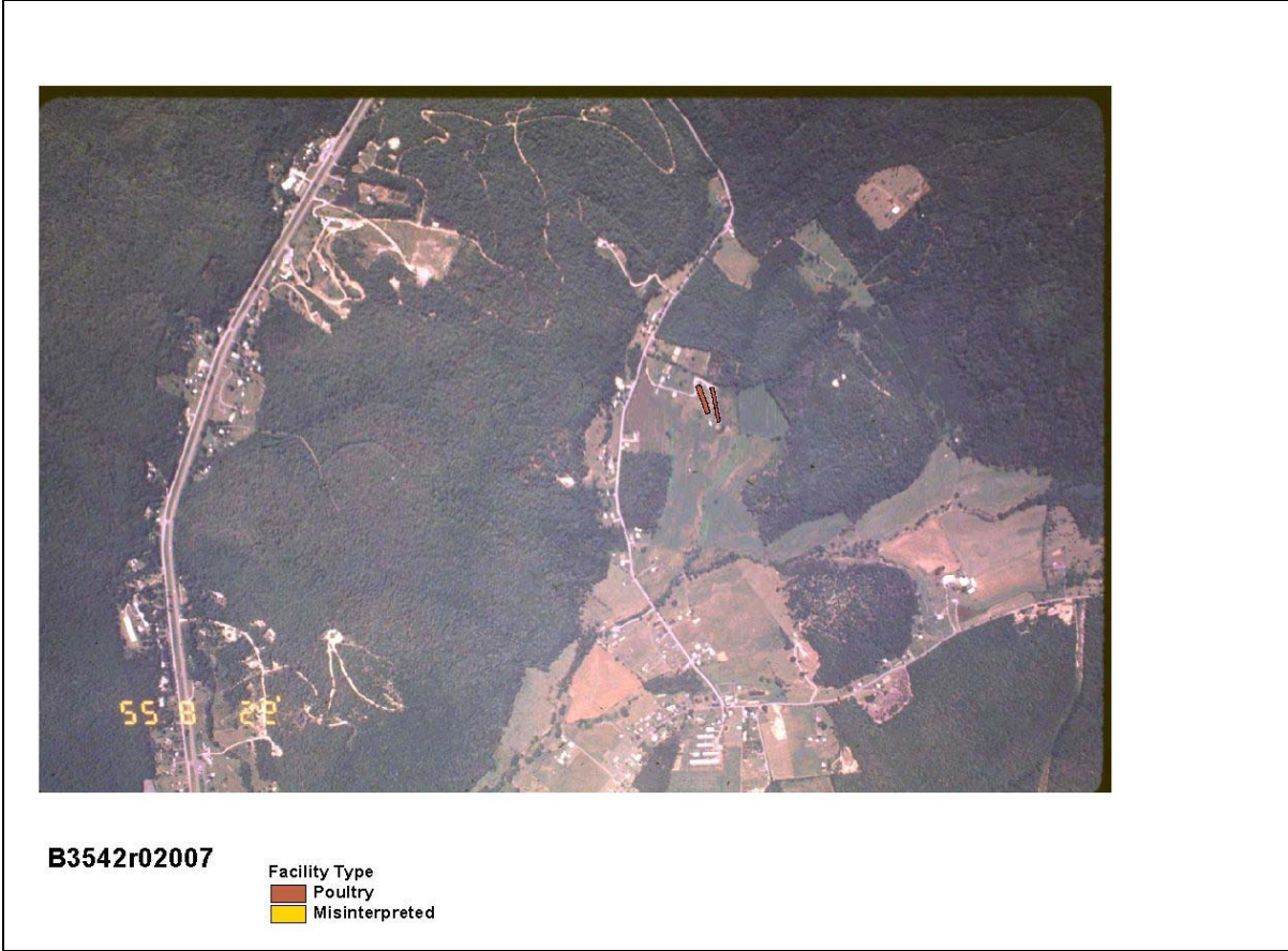
Figure A-21. Automated identification results for slide B2542r02007 (2 poultry houses identified, 0 missed, 0 misinterpreted).
