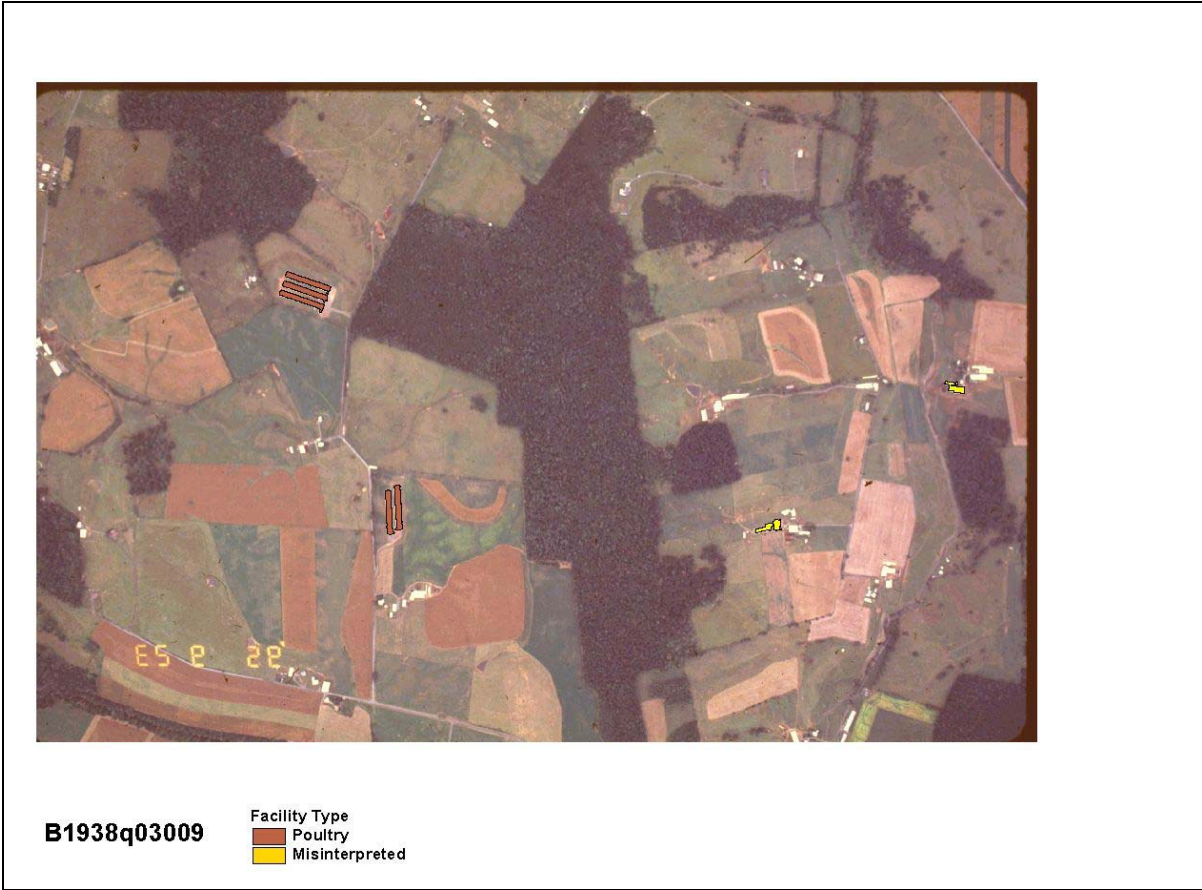
Figure A-4. Automated identification results for slide B1938q03009 (7 poultry houses identified, 0 missed, 2 misinterpreted).
