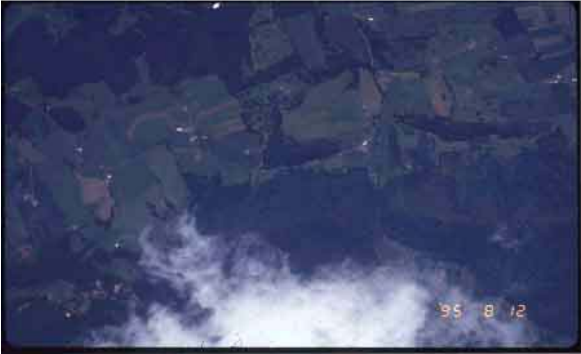
Figure 3-5. An example of a 35-mm aerial slide with significant cloud cover
