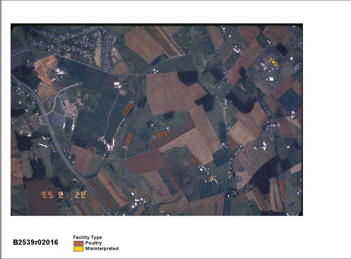
Figure A-16. Automated identification results for slide B2539r02016 (10 poultry houses identified, 0 missed, 2 misinterpreted).
