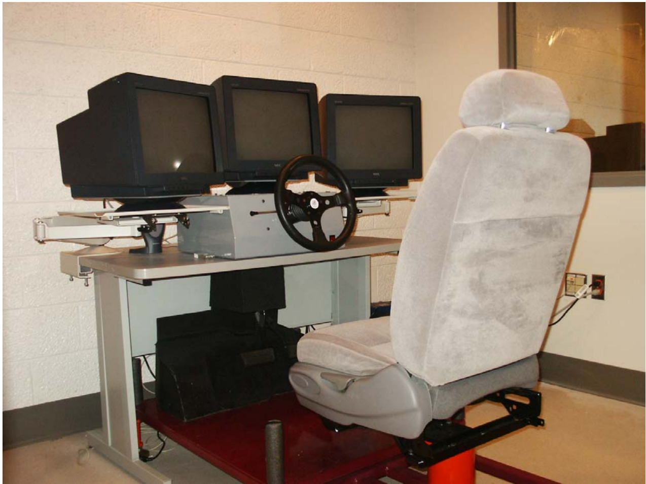
Figure 4. Picture of the STISIM Driving Simulator used in Preliminary Studies 1 & 2 and the Current Research.
