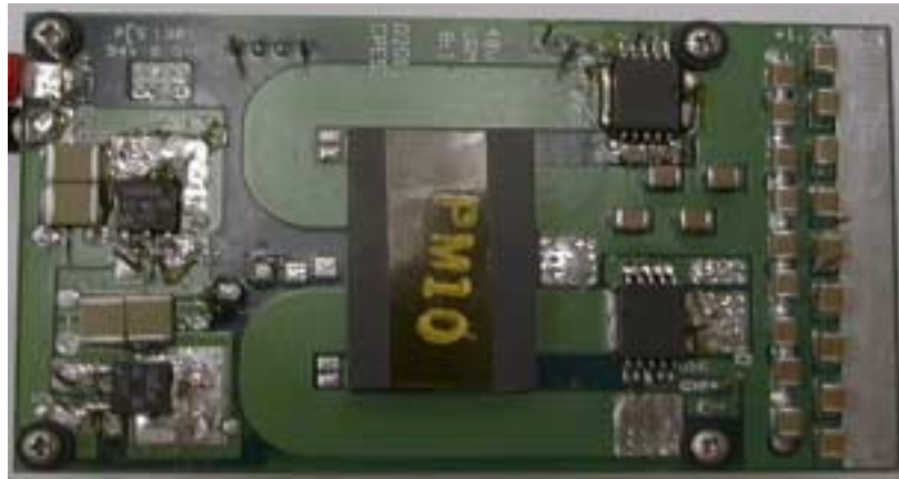
Figure 3.49. 48V VRM prototype using the single-magnetic push-pull forward converter.
