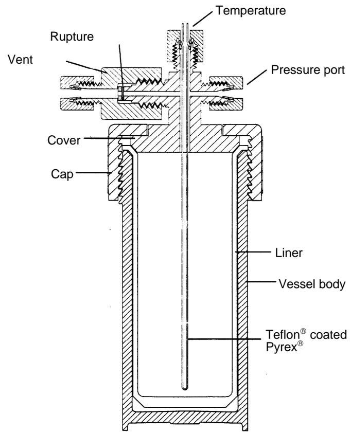
**Fig. 6 Schematic diagram of a microwave assisted extraction vessel**
