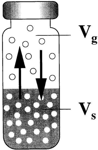
**Fig. 4 Schematic diagram of headspace vial containing a liquid sample**
