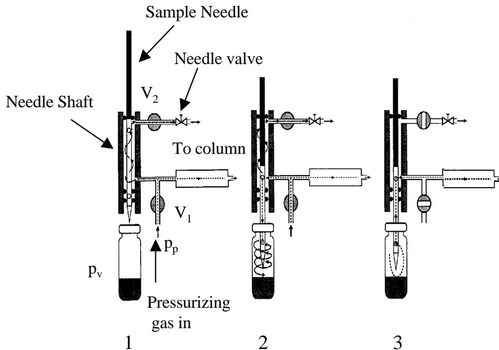
**Fig. 5 Schematic diagram of the automatic balanced pressure system <sup>(54)</sup>. (1) equilibration (stand-by), (2) pressurization, (3) sample transfer.  $V$  = on/off solenoid valves,  $p_p$  = pressurizing pressure,  $p_v$  = original headspace pressure in the vial.**
