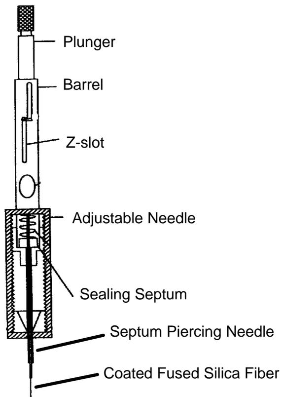
**Fig 1. Schematic diagram of SPME assembly**
