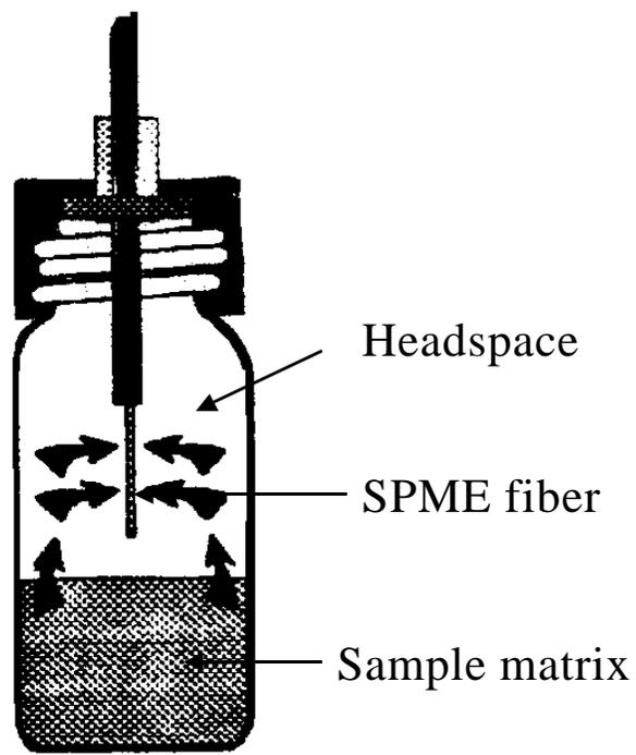
**Fig. 3 Schematic diagram of SPME-headspace**
