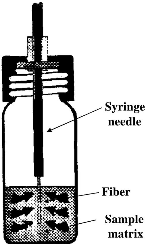
**Fig. 2 Schematic diagram of SPME absorption**
