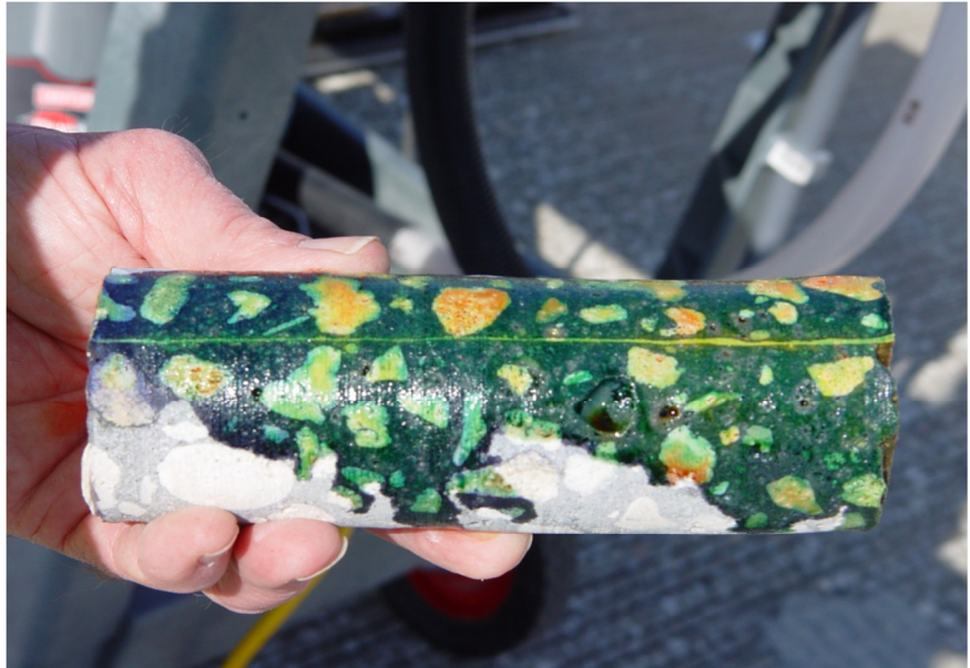
Figure 67 – pH Color Indicator Test on Concrete Cores
