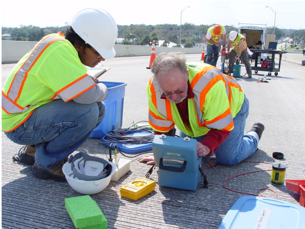
Figure 65 – Three-Electrode Linear Polarization Measurement
