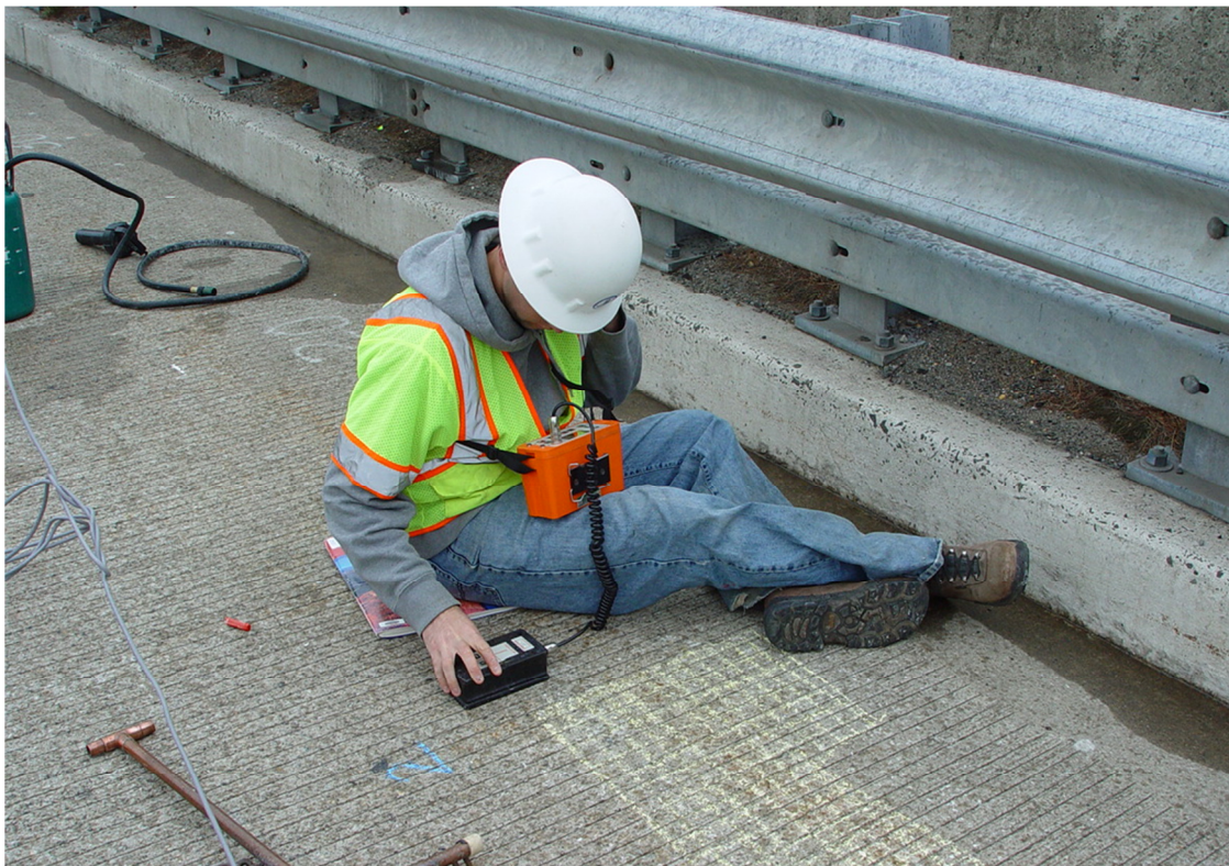
Figure 85 – Cover Depth Measurement using Pachometer
