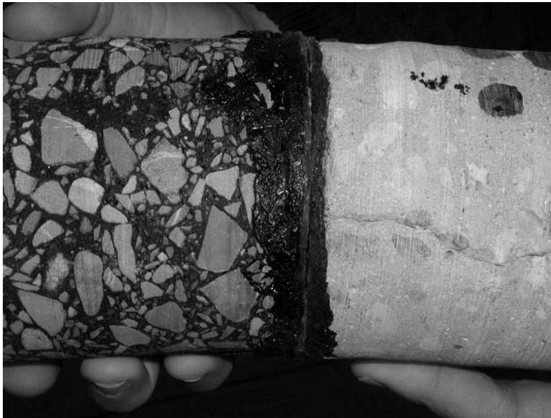
Figure 3-22. Performance of the Geocomposite Membrane in Delaying the Reflection of Cracks in a Bridge Deck in Italy
