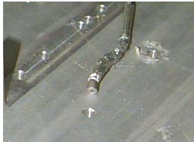
**Figure 2.27: Microphone lying beside mounting hole on interior of wing**
