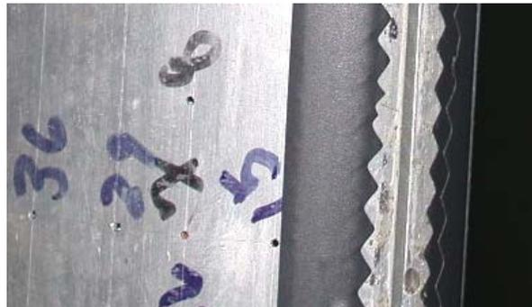
*Figure 2.33: Close-up of boundary layer trip strip*
