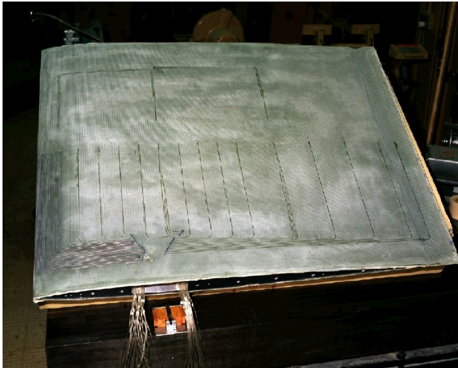
Figure 3: Model Pressure Port Layout
