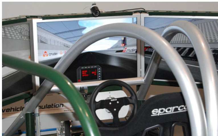
Figure 2.2: View of the virtual track used for HIL testing on the driving simulator.
