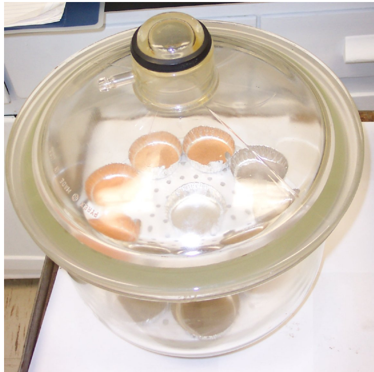
Figure 6.2 Dishes containing soil specimens placed in a desiccator for surface area measurement
