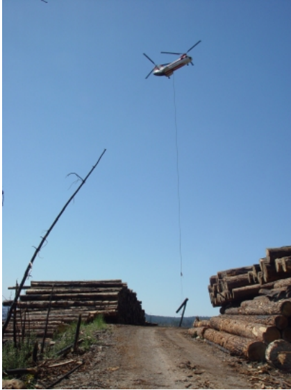
Figure 3. A helicopter is descending toward the drop zone to release the chokers and leave the logs at the landing (unhooking).
