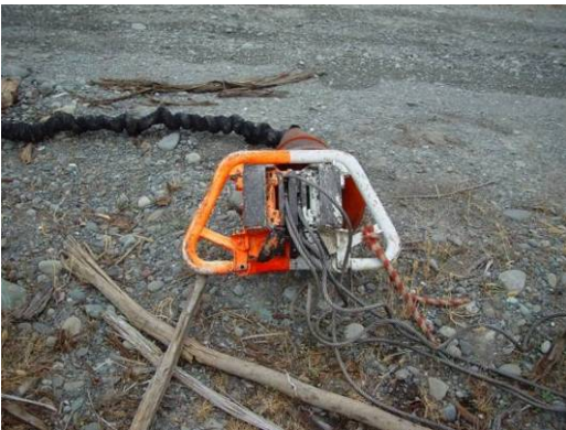
Figure 2. The underside of a hook with chokers in the slots.
