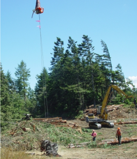
Figure 4. Coiled chokers attached to the hook are retrieved from the log landing to supply the hookers in the woods.
