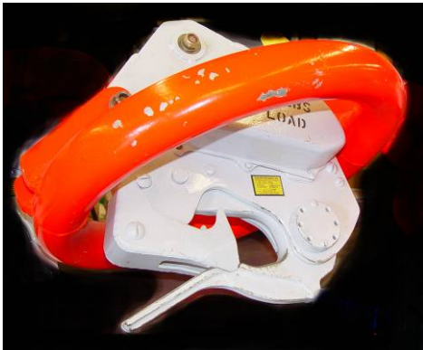
Figure 5. Helicopter hook for eyed chokers; type used prior to nubbin choker hook.
