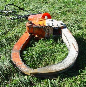
Figure 6. A grapple used for helicopter yarding.
