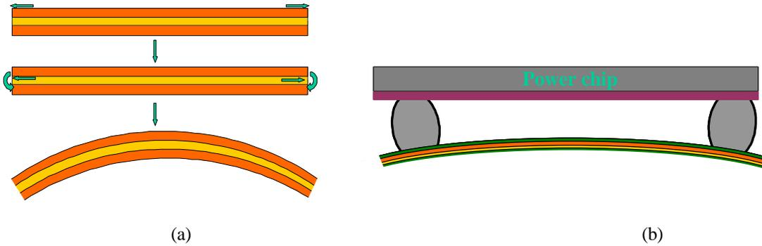
Figure 4.20. Flex buckling in flip chip on flex assembly. (a) The buckling mechanism; (b) Schematic of exaggerated thermal bending of flex substrate in flip chip on flex package.
