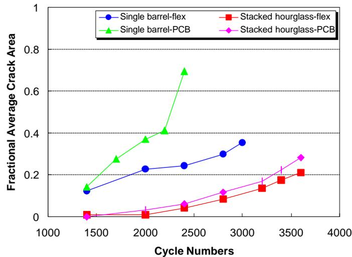
Figure 4.8. A comparison of the average crack area increase rate of FCOF and FCOB assemblies with single bump barrel-shaped solder joints and stacked hourglass/column-shaped solder joints during temperature cycling under the second temperature cycling condition.
