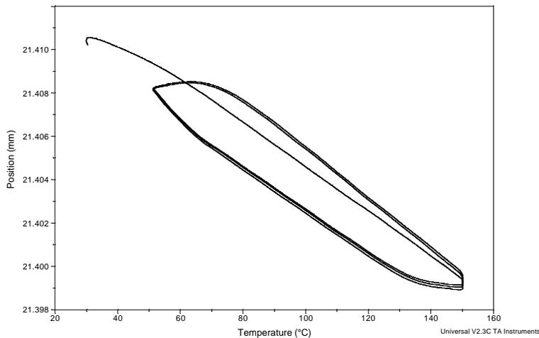
Figure 4.16. Typical TMA trace of flex displacement in a two-dimensional flex plate sample through three temperature cycles.
