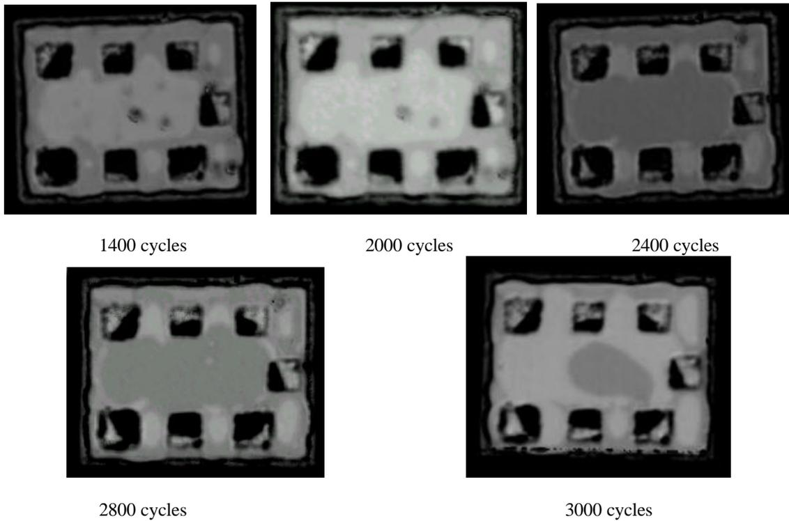
Figure 4.4. C-SAM images of the interface between single barrel-shaped solder joints and chip of a typical FCOF assembly during temperature cycling.
