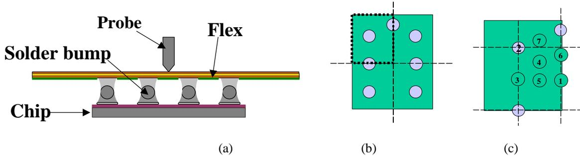
Figure 4.10. Two-dimensional flex plate test sample. (a) Cross-section view; (b) Top view; (c) Probe locations.
