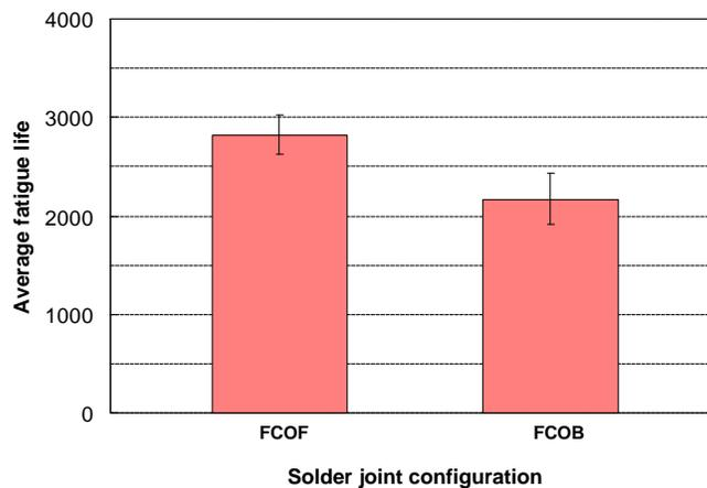
Figure 4.3. A comparison of the average fatigue life of flip chip on PCB board and flip chip on flex assemblies with single bump barrel-shaped solder joints under the second thermal cycling condition.
