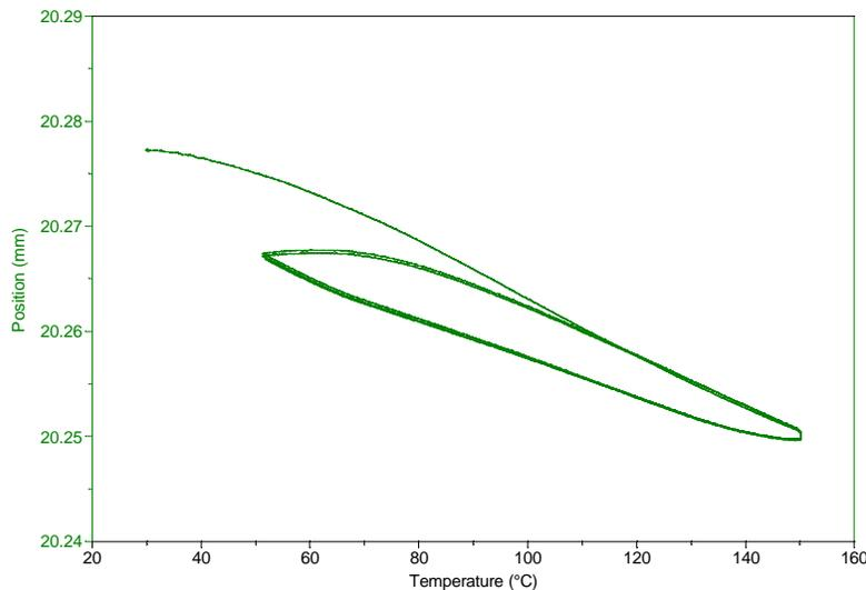
Figure 4.13. Typical TMA trace of flex displacement in one flex strip sample through three temperature cycles.
