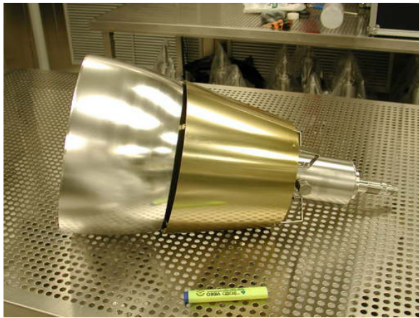
Figure 3.25: Side-view of a Borexino PMT with light concentrator and \mu -metal shielding attached
