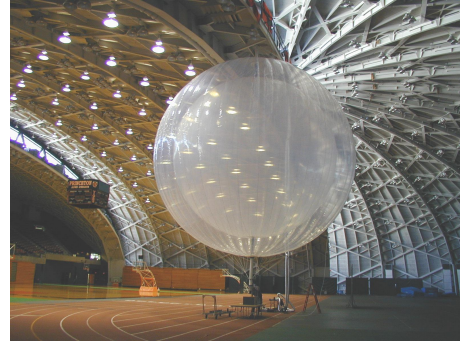
Figure 3.15: Prototype inner and outer vessels undergoing a test inflation in the Jadwin Gymnasium at Princeton University.
