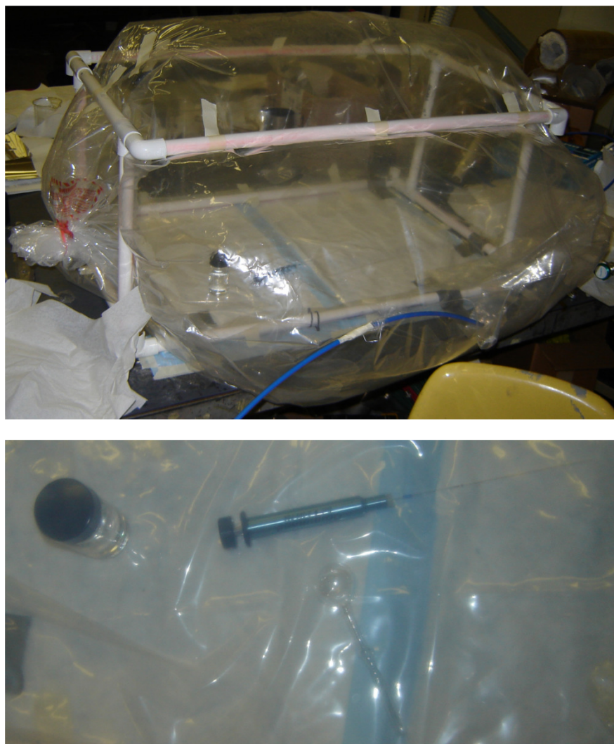
Figure 7.11: Top: The disposable glove-bag inside of which the ^{14}\text{C} -Toluene solution was loaded into the vials. Bottom: The bottle containing the concentrated ^{14}\text{C} -Toluene solution, the 100\ \mu\text{L} pipette, and the source vial.
