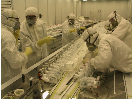
Figure 3.14: Photo taken during the construction of the vessels for Borexino. The vessels were constructed from tear shaped panels, glued and clamped together — the IV was then nested inside of the OV prior to sealing the last OV panels. John Bahcall (middle person on the left side of the table) can be seen on a visit to the cleanroom where the construction was taking place.
