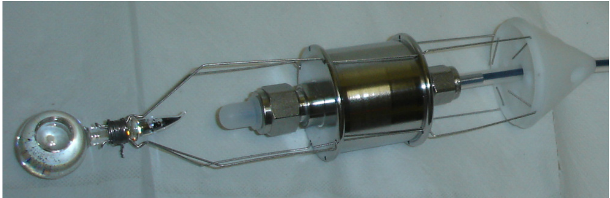
Figure 8.2: The hardware used for the on-axis test in the CTF. From right to left: cone to guide the assembly back into the fill pipe, counterweight, diffuser, and source vial. When used in Borexino, the diffuser was replaced with another source vial filled with glass beads.
