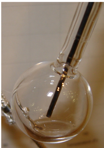
Figure 7.13: A closeup view of a ^{14}\text{C} - ^{222}\text{Rn} source just before radon loading. The exhaust tube can be seen here just above the bottom of the vial where a small pool of the ^{14}\text{C} solution has been placed. After immersing the vial in liquid nitrogen, radon loaded nitrogen flows down through the neck of the vial, and freezes out onto the surface of the vial, and the excess gas flows up the exhaust tube and to a fume hood. Before sealing the vial, the exhaust tube is withdrawn up to a level above the sealing point of the vial.
