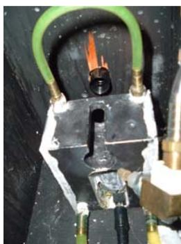
**Figure B. 5. Cylindrical Quartz Sample Cell, Part Number 14-385-930E**
