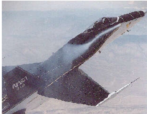
Figure 1.1: Flow visualization of leading-edge extension vortex burst, 30^\circ angle of attack (Photograph Courtesy of the NASA Dryden Flight Research Center)
