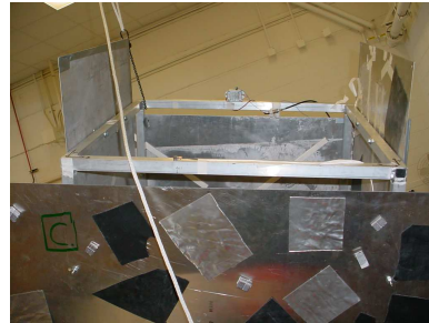
(c) External disturbance actuator oriented in the vertical axis on top of the structure
