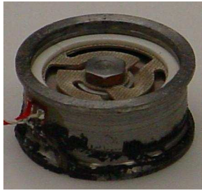
Figure 3.15 Actual electromagnet shaker characterized.
