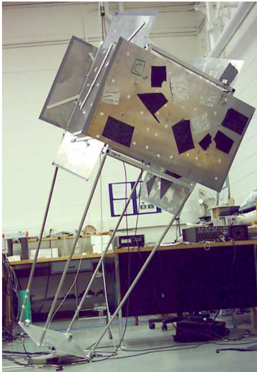
(a) Complete structure suspended by elastic cord at a single point
