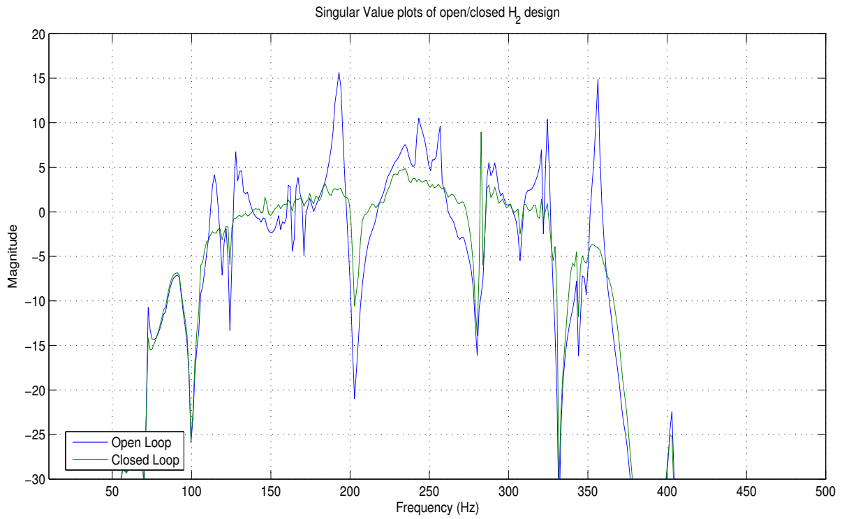
Figure 4.18 Low-frequency H_2 example performance singular values
