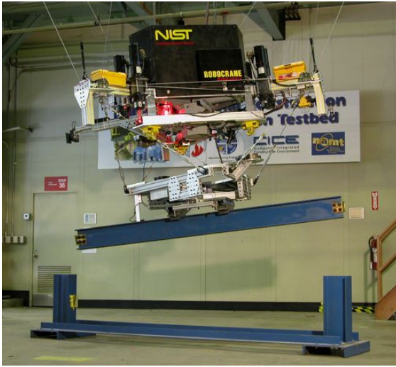
(a) The NIST RoboCrane transporting the test beam to the dock position
