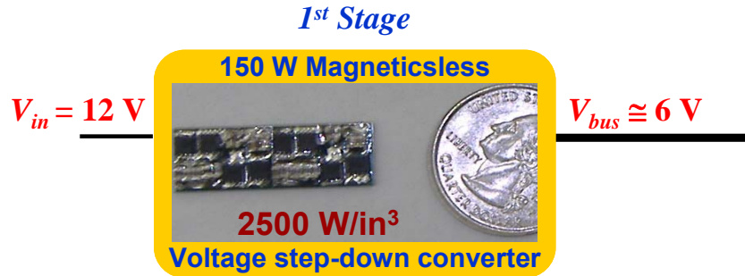
Figure 5.17. First stage in a 2-stage conversion concept for VRM and other high power applications [113].
