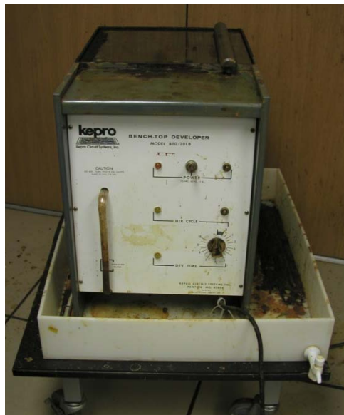
Figure 3.23. Kepro wet etcher used to remove copper from the DBC.
