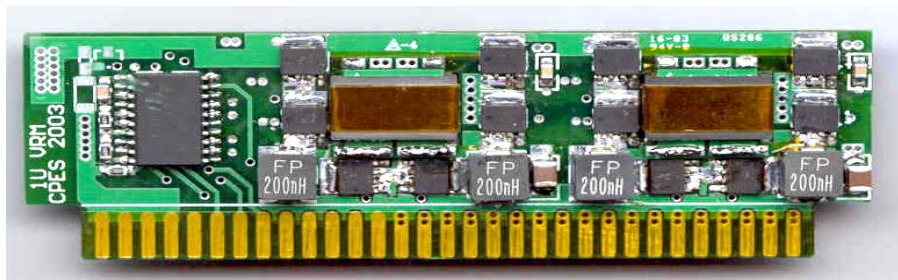
Figure 2.1 CPES-designed 1 MHz self-driven VRM in 1U form factor [82]
