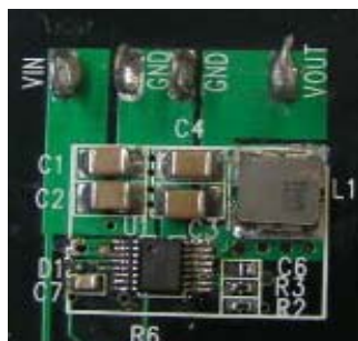
Figure 1.14. Typical use of PCB substrate with all the components mounted on top, preventing layering of substrates.
