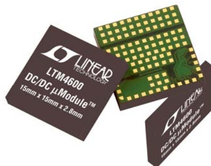
Figure 1.8. Linear Tech LTM4600 module with all components co-packaged together. Backside pad interconnections are also shown.
