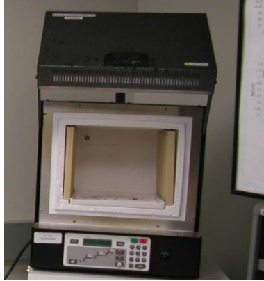
Figure 3.25. Programmable oven for curing the epoxy. Shown with the front door open (it opens upwards).
