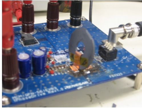
Figure 4.4. LTCC 1-turn inductor in buck circuit for characterization.
