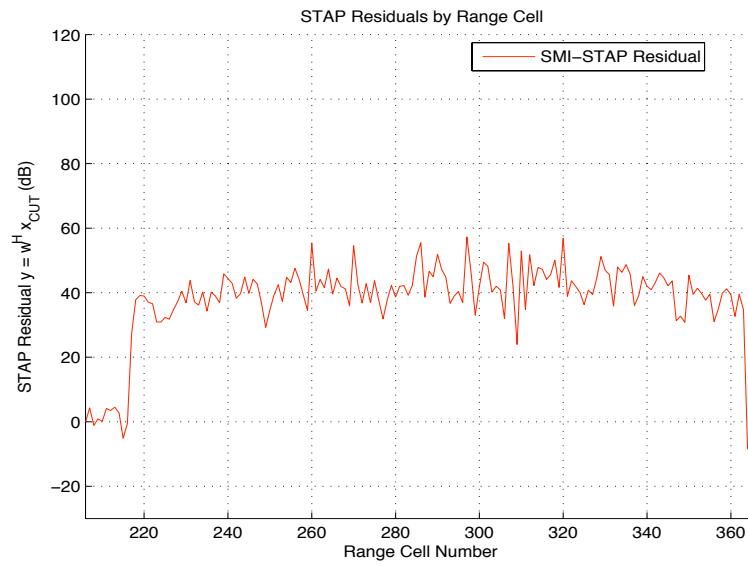
Figure 4.19: STAP residue performance vs. range cell with no NHD used. No reliable detection of targets.
