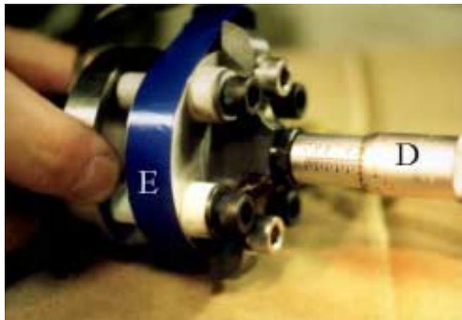
Figure 2.4: The Micrometer Drive Assembly
