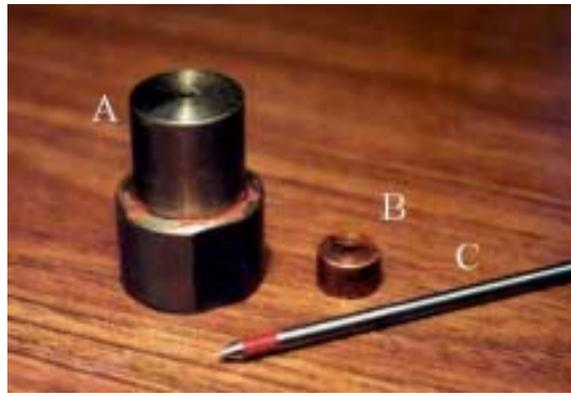
Figure 2.2: Plasma Torch Electrodes
