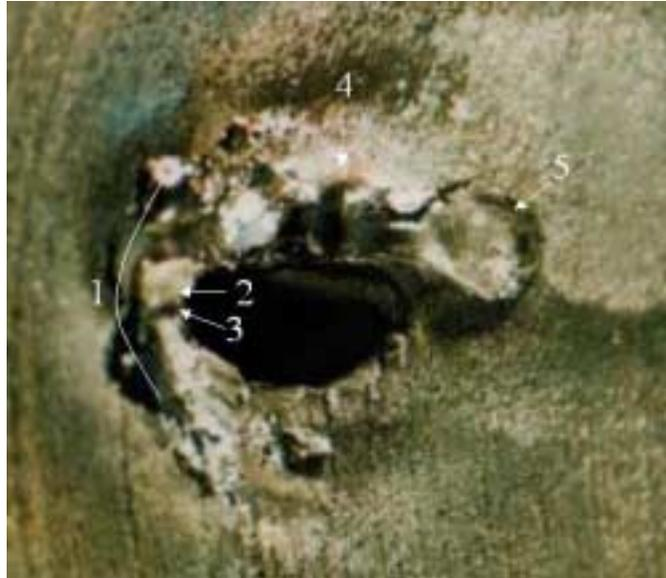
Figure 6.26: Anode Wear on the 60°, 2.54-mm Throat Length, Sonic Anode
