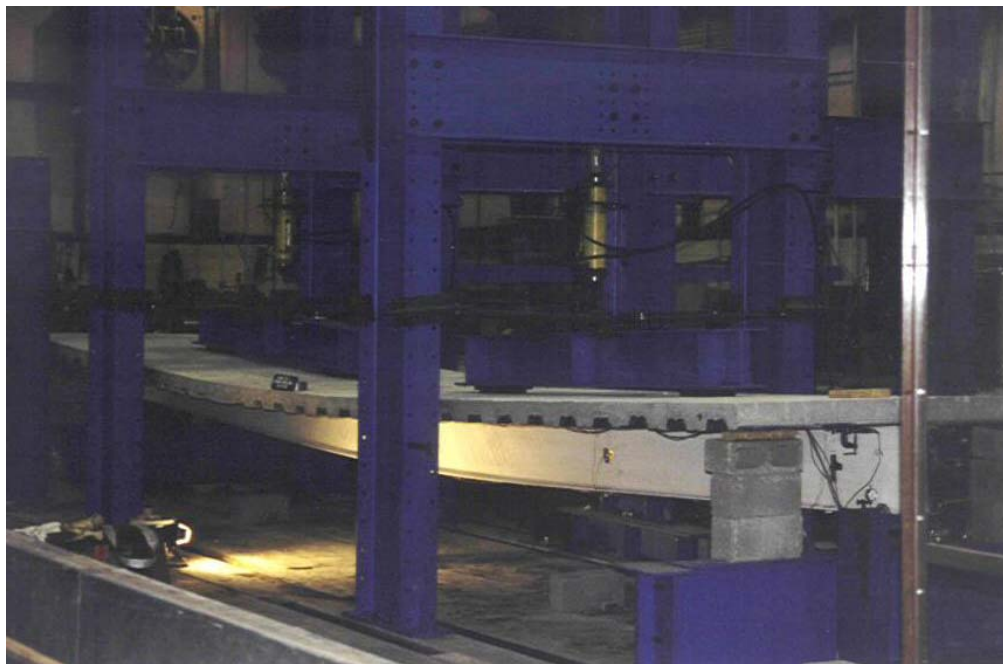
Fig. 7.6 Beam Test 1 Showing Large Deflections
