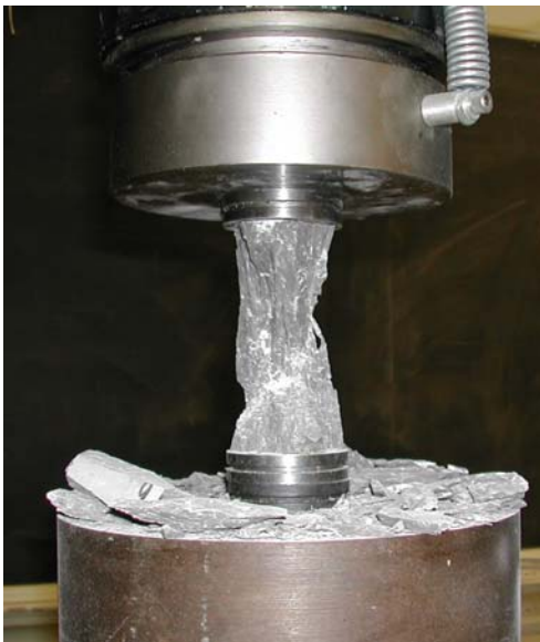
FIGURE 3.2 SAMPLE AFTER BEING CRUSHED IN THE UNIAXIAL COMPRESSIVE TESTING MACHINE.
