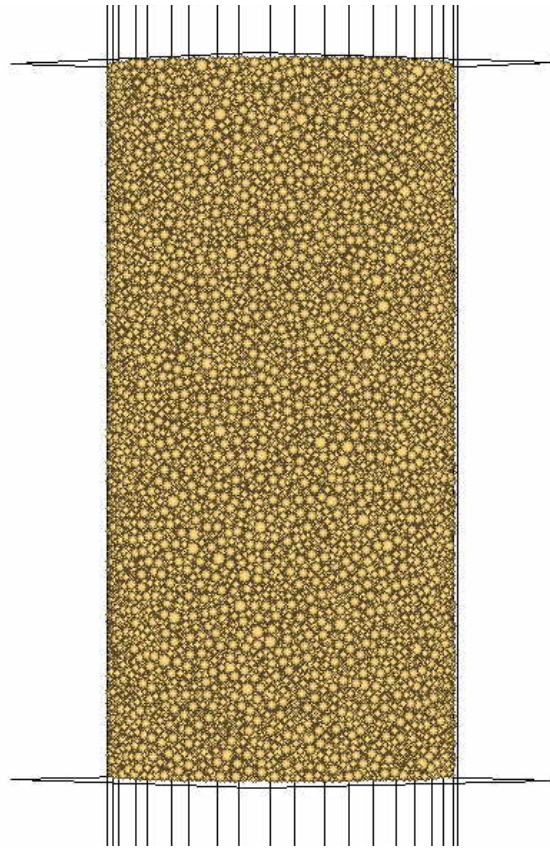
FIGURE 4.4 INITIAL MODEL USED IN PFC 3D ALONG WITH THE FLAT PLATENS FOR THE VALIDATION PROCESS.
