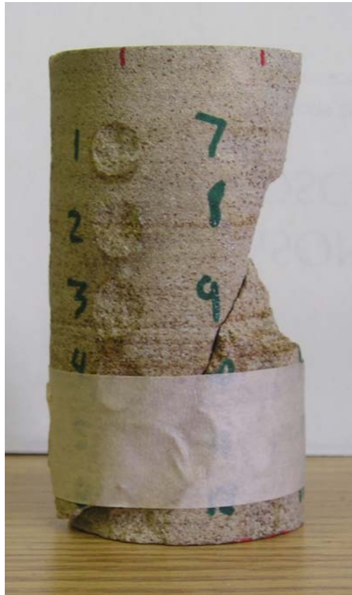
FIGURE 6.12 BEREA SANDSTONE AFTER FAILURE
