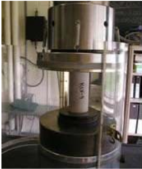
FIGURE 3.1 SAMPLE IN THE UNIAXIAL COMPRESSIVE TESTING MACHINE.
