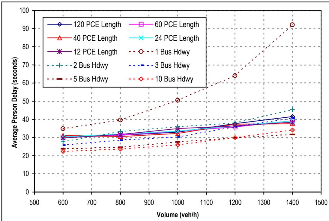
Figure 7.10: Comparison of Average Person Delay Estimates between Scenario 2 and 3
