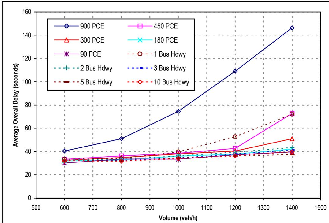
Figure 7.12: Comparison of Average Overall Delay Estimates between Scenario 2 and 4
