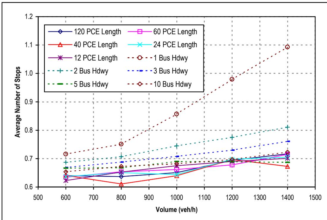
Figure 7.11: Comparison of Average Number of Stops between Scenario 2 and 3
