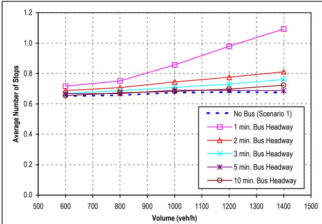
**Figure 7.8: Comparison of Average Number of Stops between Scenario 1 and 2**
