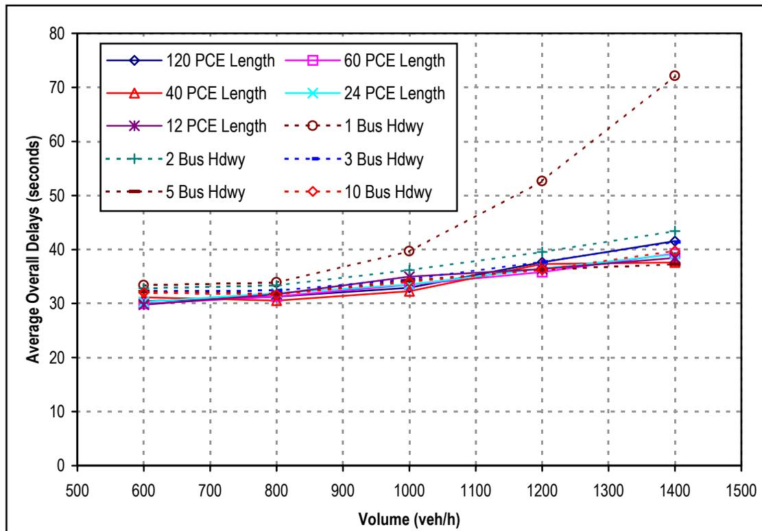
**Figure 7.9: Comparison of Average Overall Delay Estimates between Scenario 2 and 3**
