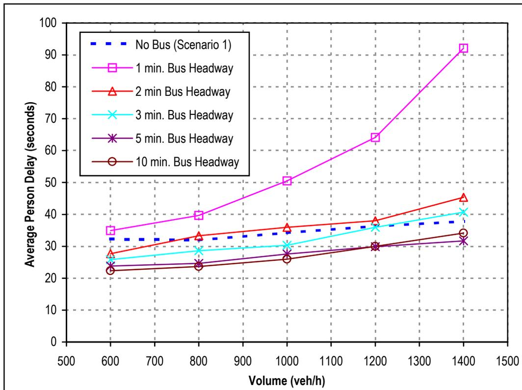
**Figure 7.6: Comparison of Average Person Delay Estimates between Scenario 1 and 2**
