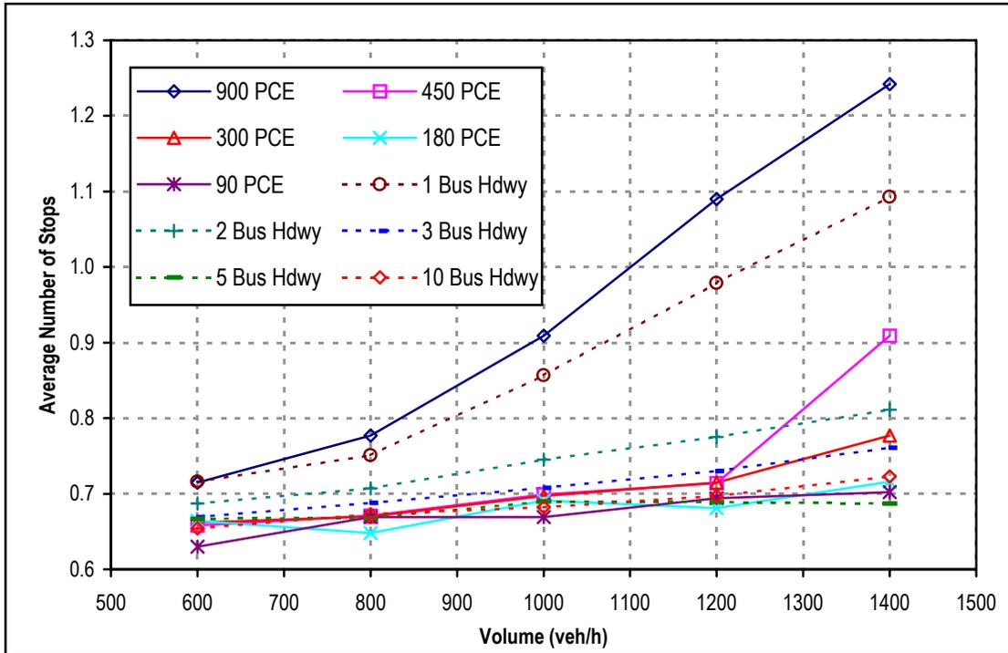
**Figure 7.14: Comparison of Average Number of Stops between Scenario 2 and 4**
