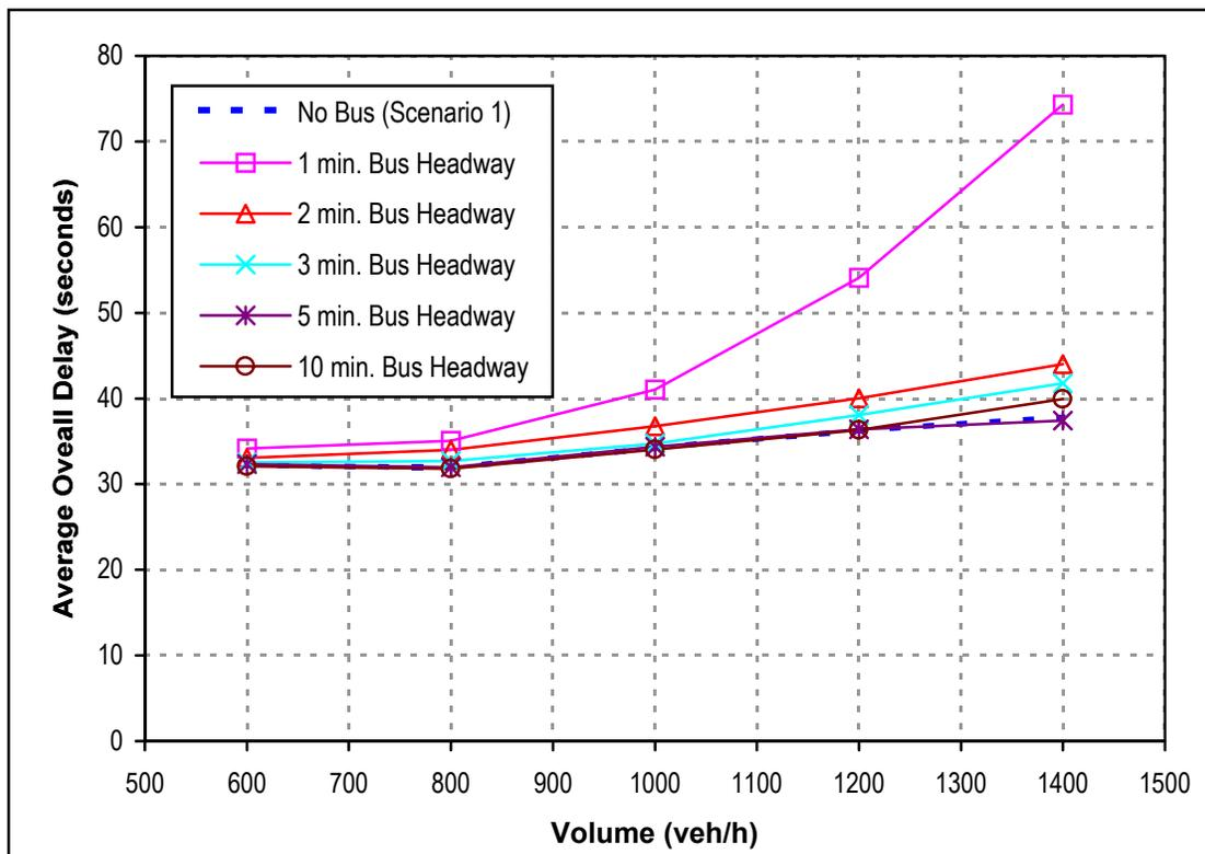
**Figure 7.4: Comparison of Average Overall Delay Estimates between Scenario 1 and 2**
