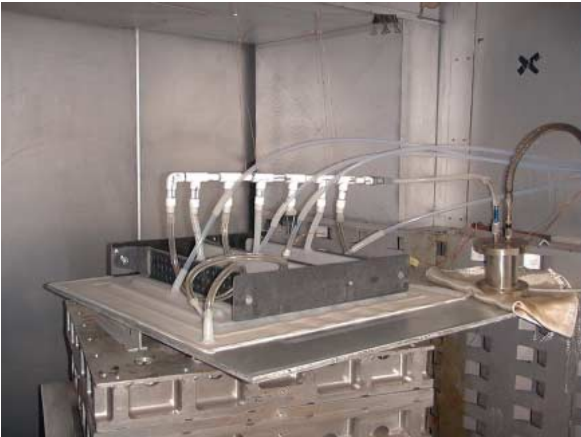
Figure 5.8 Experimental VARTM Processing Set-Up for a Three-Stiffener Carbon Panel
