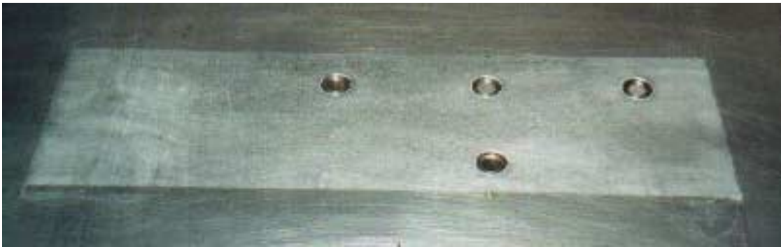
Figure 3.3 VARTM In-Plane Fixture for Advancing Front Permeability Measurements
