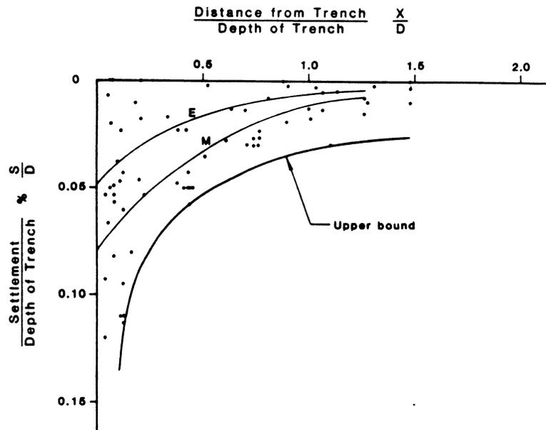
Figure 2.7 Ground Settlement Due to Slurry Trench Excavation (Cowland and Thorley 1985)
