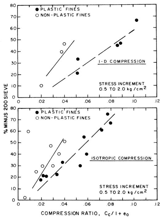
Figure 2.2 Compression Ratio Versus Fines Content for Various Soil-Bentonite Mixtures (D'Appolonia 1980)
