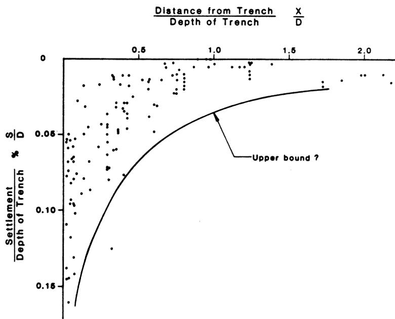
Figure 2.8 Building Settlements Due to Slurry Trench Excavation (Cowland and Thorley 1985)
