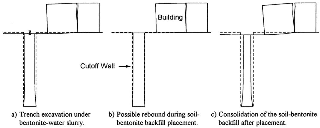
Figure 2.6 Ground Deformations Due to Construction of a Soil-Bentonite Cutoff Wall (Filz 1996)
