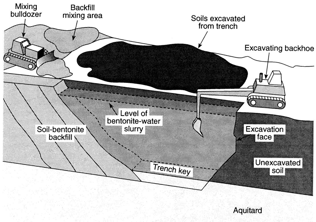
Figure 2.1 Soil-Bentonite Cutoff Wall Construction Process (*Barrier 1995*)
