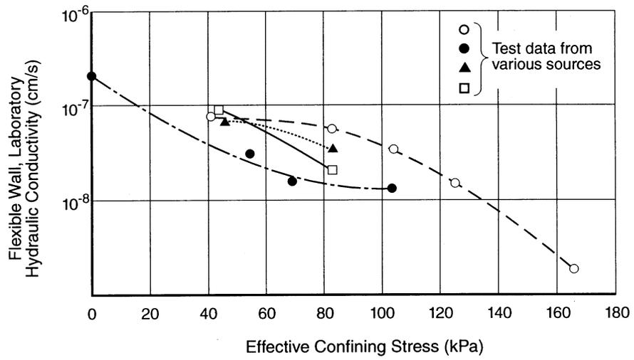
Figure 2.4 Effect of Consolidation Pressure on Hydraulic Conductivity of Soil-Bentonite Mixtures (*Barrier 1995*)
