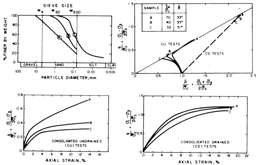
Figure 2.3 Triaxial Test Data on Various Soil-Bentonite Mixtures (D'Appolonia 1980)
