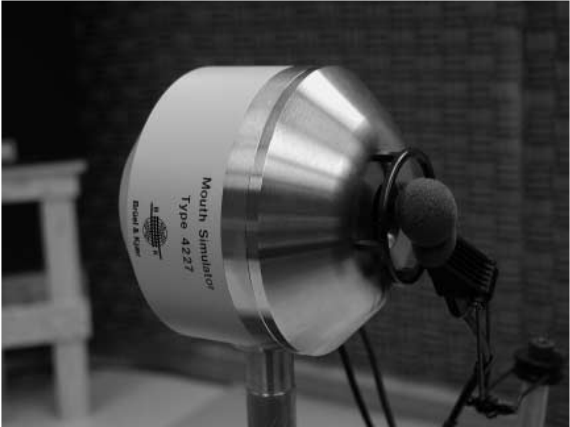
Figure 18. The Gentex communication microphone in front of the artificial mouth.
