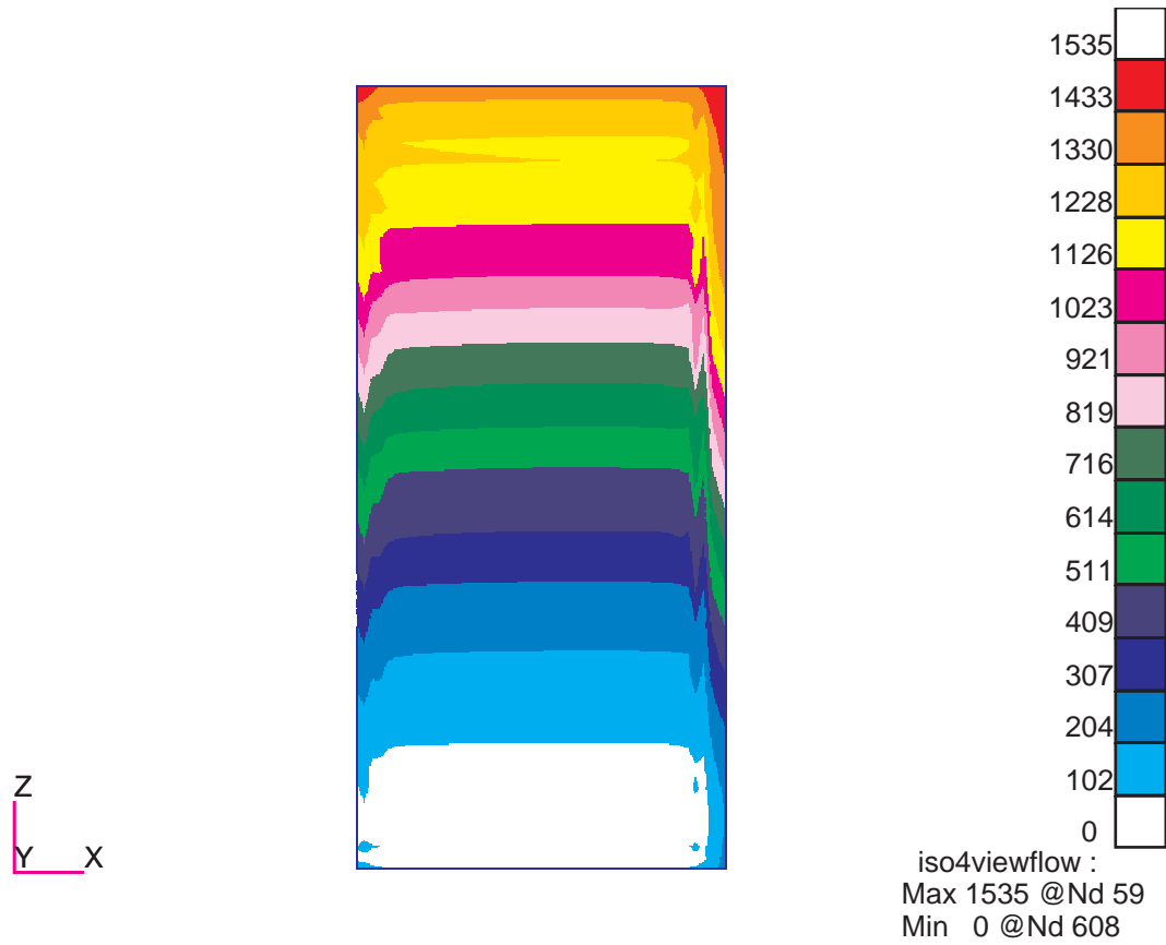
Figure 6.52: Predicted flow front progression in the bottom surface of the stitched foam core preform with 6.35 mm stitch row spacing
