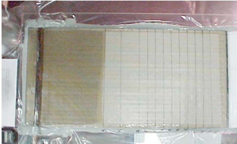
Figure 6.19: Top surface of stitched foam core preform with 12.7 mm stitch row spacing. Flow front is approximately 25.4 cm from injection edge
