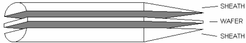
The Split Billet Assembly for Solid State Coextrusion of Films
