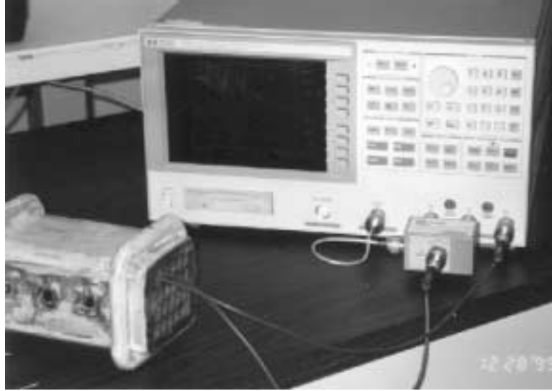
Figure B.2: Sample Coil Connected to the Network Analyzer
