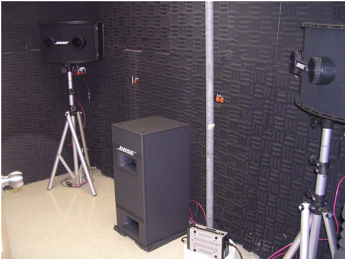
Figure 18. Speaker system which produced the Cessna engine noise inside the flight simulator room.
