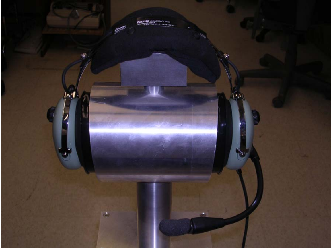
Figure 20. Acoustical test fixture used to measure protected exposure levels without communications (ANSI S12.42-1995).
