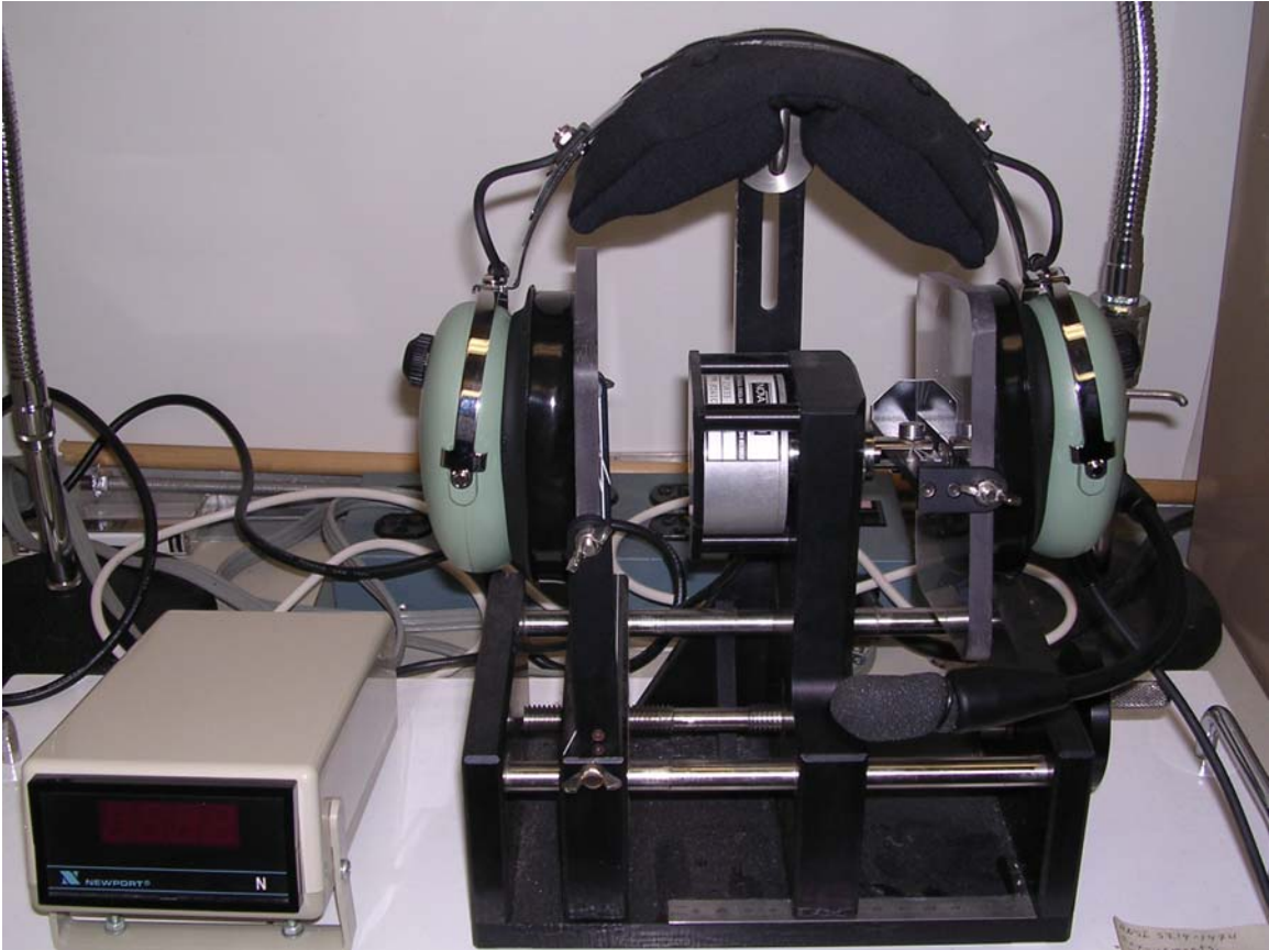
Figure 21. Headband clamping force measurement device (ANSI S3.19-1974).
