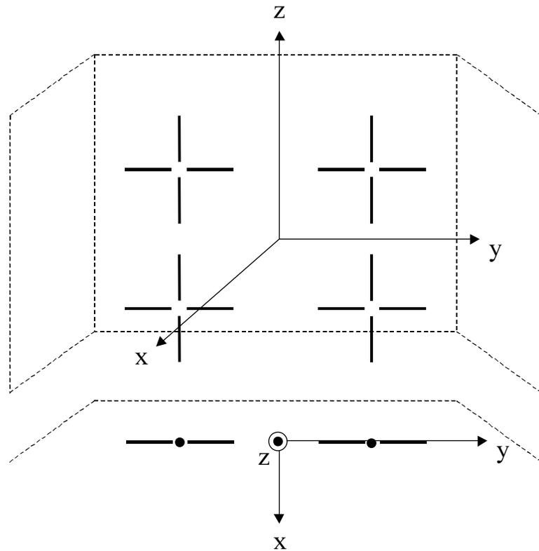
**Figure 5-5.** The multi-polarized adaptive array investigated in [5.9]
