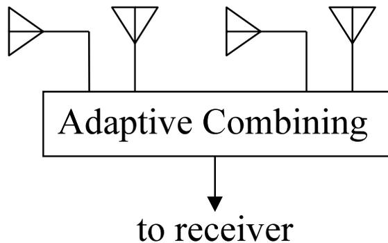
**Figure 5-2.** A multi-polarized adaptive array
