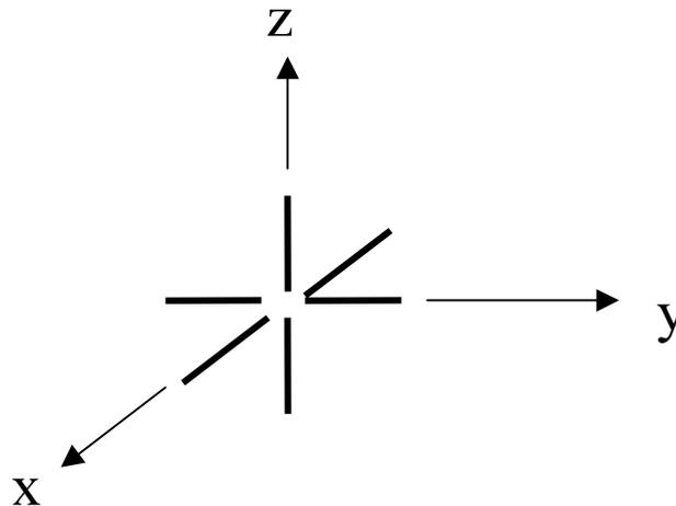
**Figure 5-4.** The “tripole” array [5.2]
