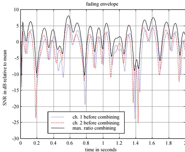
**Figure 7-12.** Fading envelopes of the signals before and after maximal ratio combining
