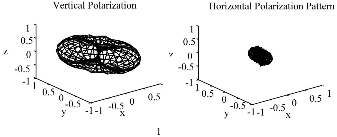
**Figure 7-8.** Pattern of a half-wave dipole that has been rotated by  $20^\circ$  from vertical
