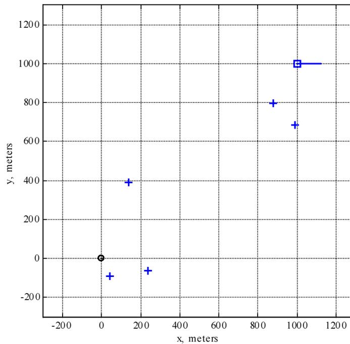
**Figure 7-11.** Diversity Simulation, location of transmitter, receiver, and scatterers
