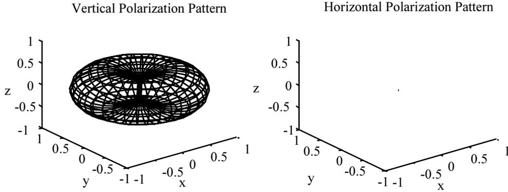
**Figure 7-6.** Sampled 3-dimensional pattern of a vertical half-wave dipole with  $10^\circ$  resolution in  $\theta$  and  $\phi$ . The pattern has no horizontally polarized component.
