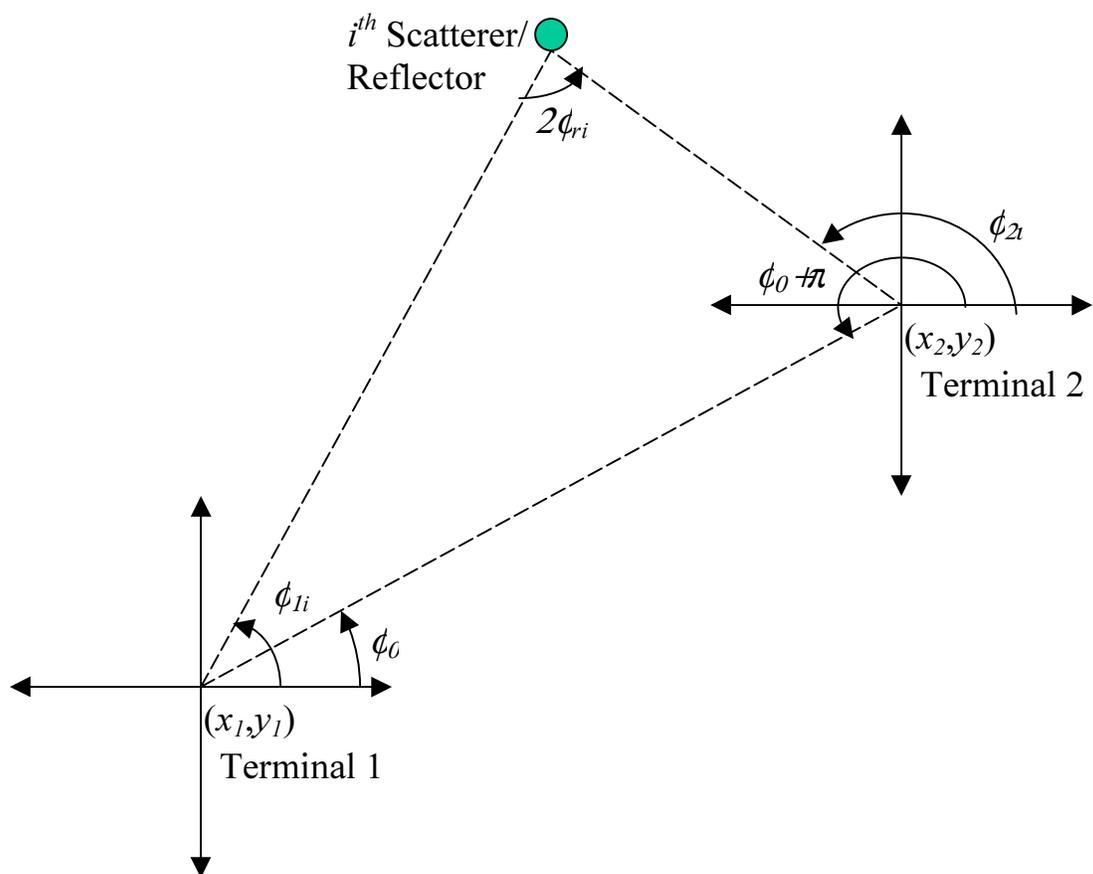
**Figure 7-9.** Geometry of link with multipath reflection for VMPS
