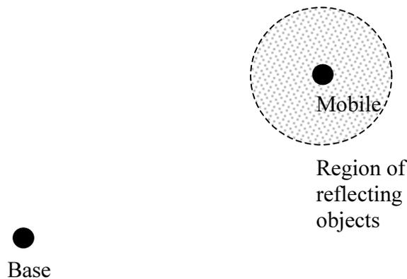
**Figure 7-2.** Geometrically-based single-bounce circular model
