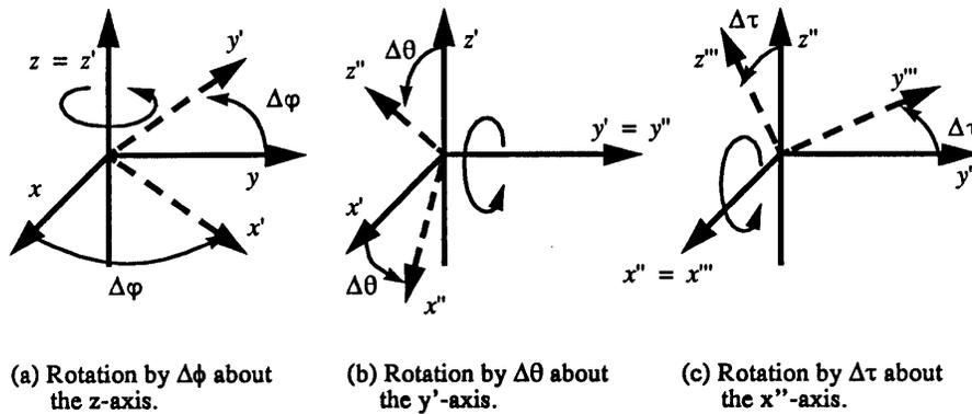
**Figure 7-7.** A three step rotation procedure that provides the ability to point the antenna in an arbitrary direction. The rotated pattern is referred back to the original coordinate system [7.7]
