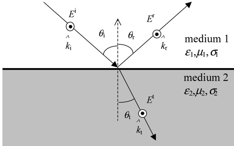
**Figure 7-4.** Reflection and transmission of polarized wave (perpendicular polarization shown)
