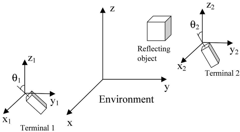
**Figure 7-5.** Coordinate systems for modeling transmission and reception of polarized waves
