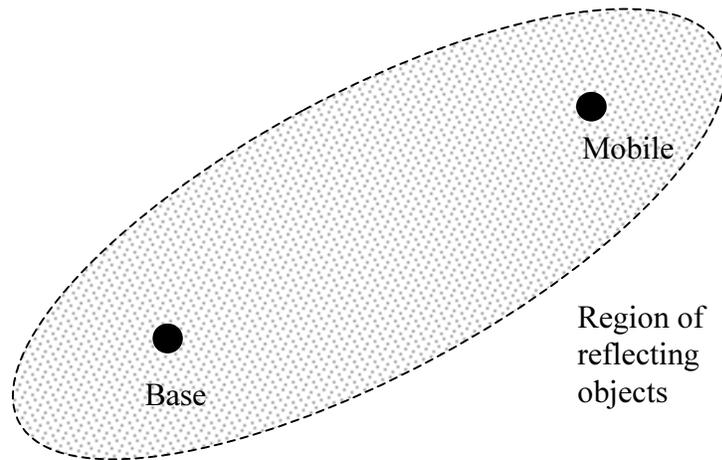
**Figure 7-3.** Geometrically-based single-bounce elliptical model
