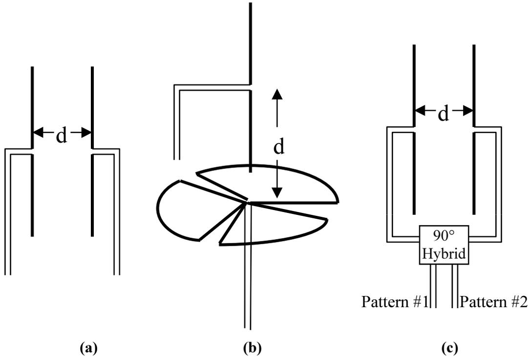
**Figure 8-3.** Diversity antenna configurations: (a) spatial, (b) polarization, (c) pattern
