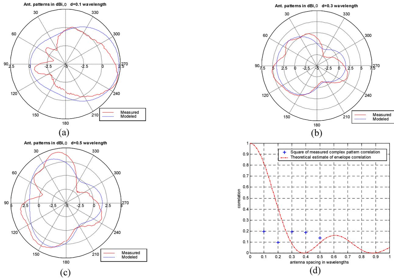
**Figure 8-4.** Effects of mutual coupling: (a) azimuth pattern of dipole with  $0.1\lambda$  spacing, (b) azimuth pattern of dipole with  $0.3\lambda$  spacing, (c) azimuth pattern of dipole with  $0.5\lambda$  spacing, (d) squared correlation of complex pattern vs. spacing, measured and theoretical for omnidirectional patterns.
