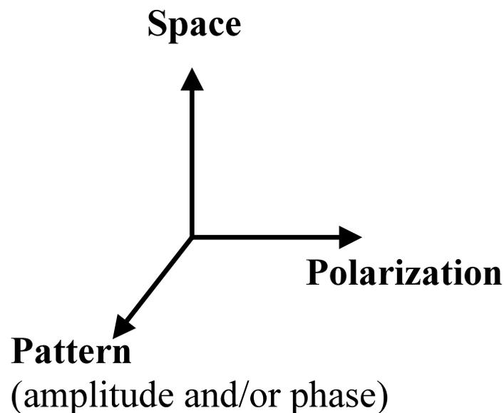
**Figure 8-1.** Three “dimensions” of antenna diversity
