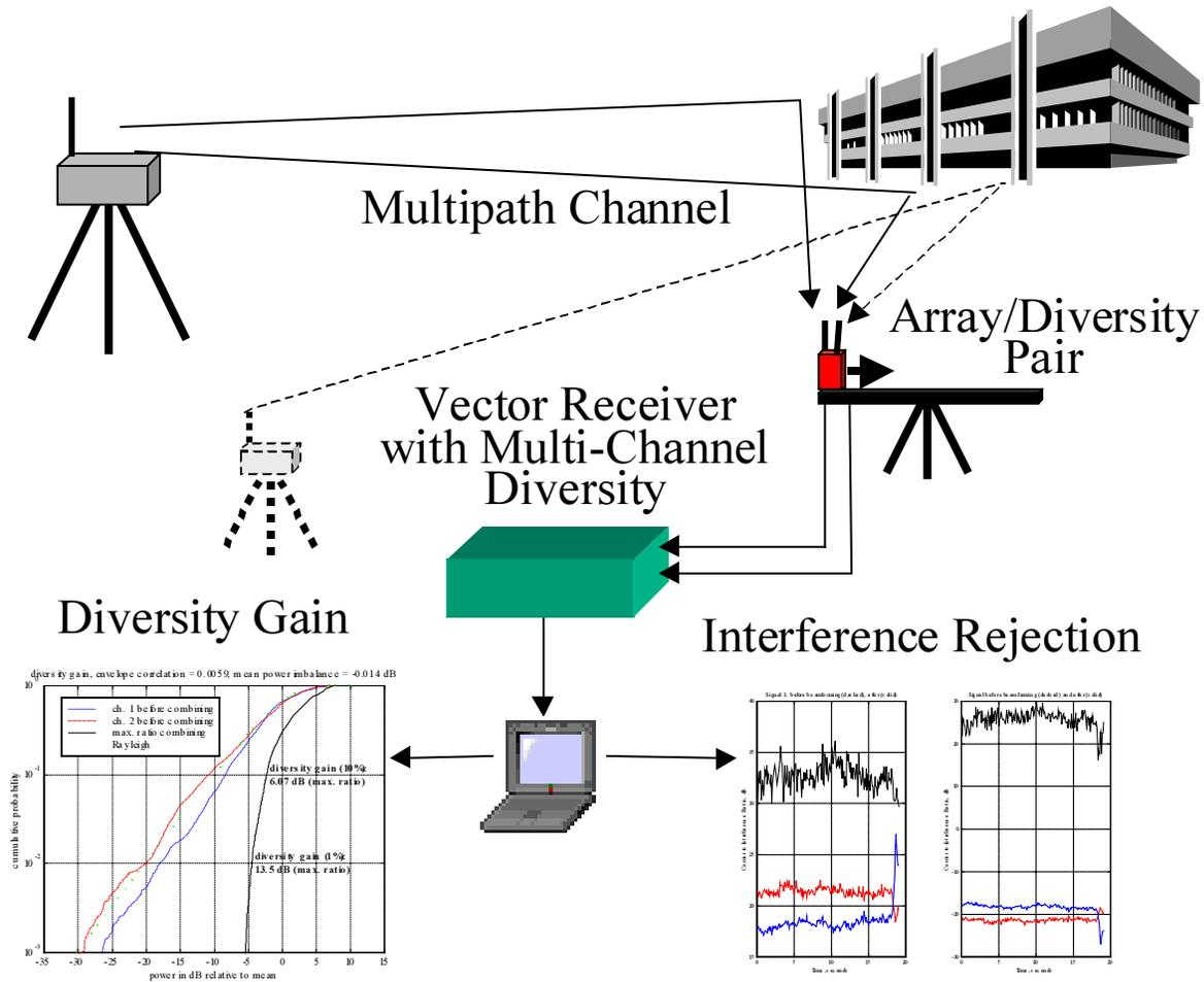
**Figure 8-2.** Overview of the Handheld Antenna Array Testbed (HAAT)
