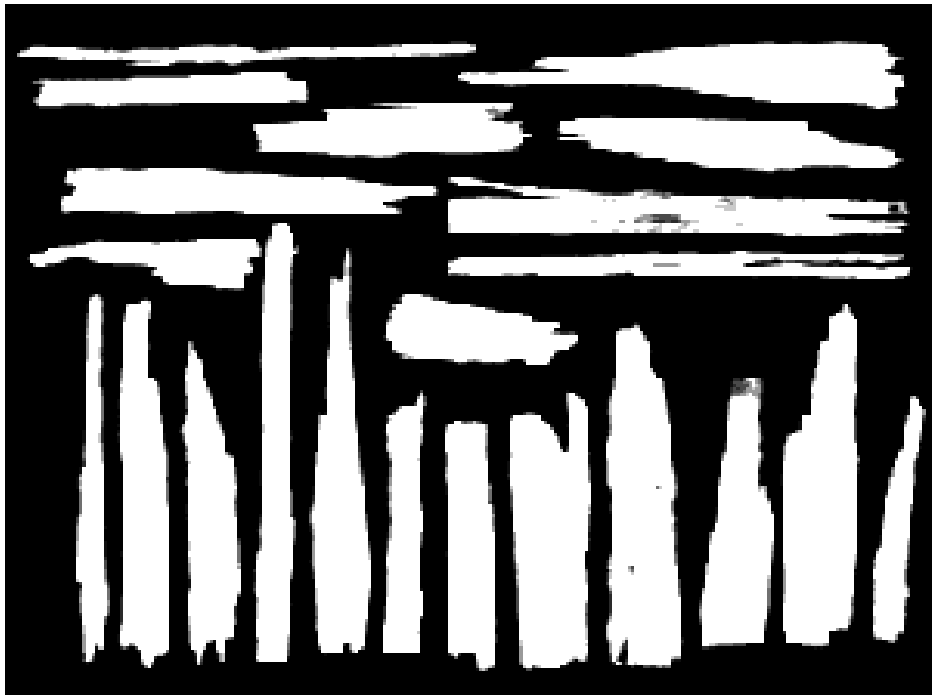
Figure 2.6. Typical digital image of face layer strands captured by the image analysis system.
