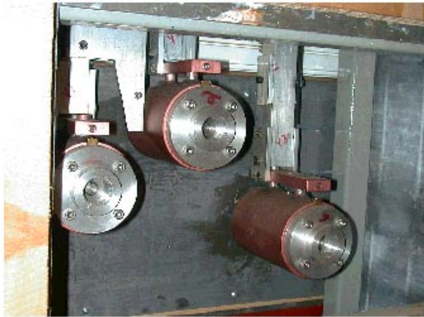
Figure 6.1. The relative positions of the \gamma -ray sources mounted on the side of the hot press.
