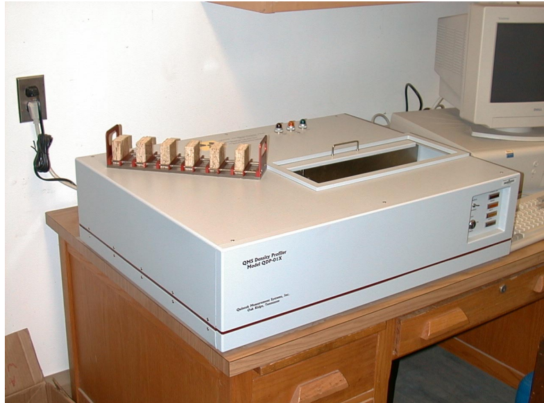
Figure 6.2. The QMS x-ray density profiler.
