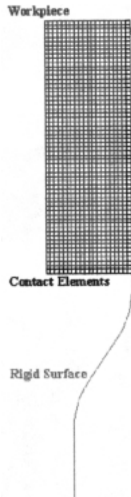
Figure 46: The finite element model mesh used in the simulation of codeformation via extrusion.
