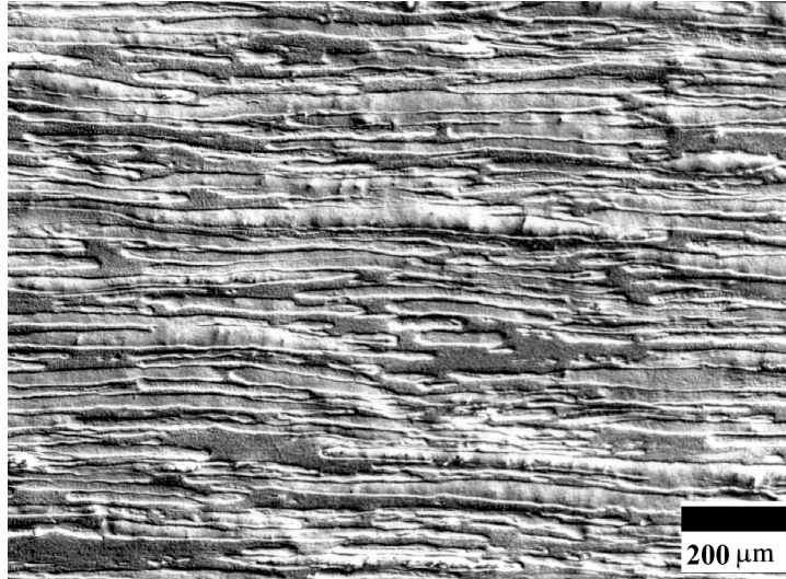
Figure 42: A micrograph of an as-polished and etched transverse cross-section taken from the center of the Ti-6Al-4V + 40 v% \text{Al}_3\text{Ti} extrusion. The \text{Al}_3\text{Ti} is shown as the darker gray component and is co-continuous with the Ti-6Al-4V component (lighter gray).
