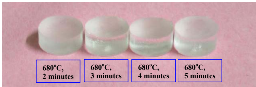
Figure 5.32: LS_2 glass samples heat-treated conventionally at 680°C for 2, 3, 4, and 5 minutes, respectively.
