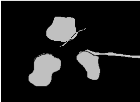
Figure 9-3 Water Invades the Interface – Stripping
