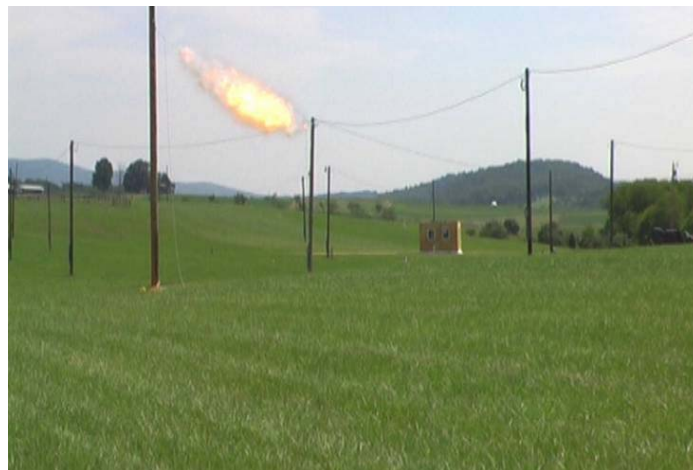
Figure 3.22: Picture of linear charge distribution being detonated.
