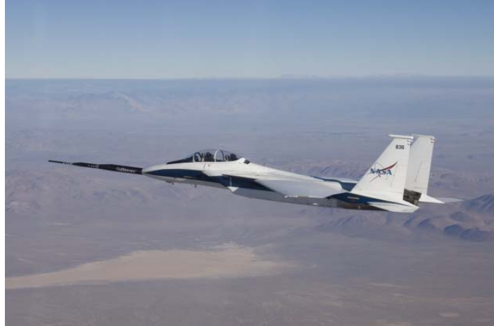
Figure 1.5: Photograph of an F-15B in flight with quiet spike attached [21] (fair use).
