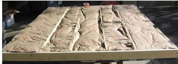
Figure 3.2: a) Plaster-wood wall instrumented with microphones and installed in the cinderblock room, and b) wall frame with insulation.
