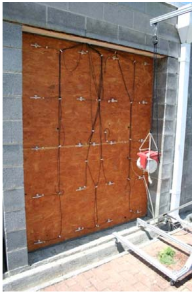
Figure 3.6: Experimental setup of the modal test.
