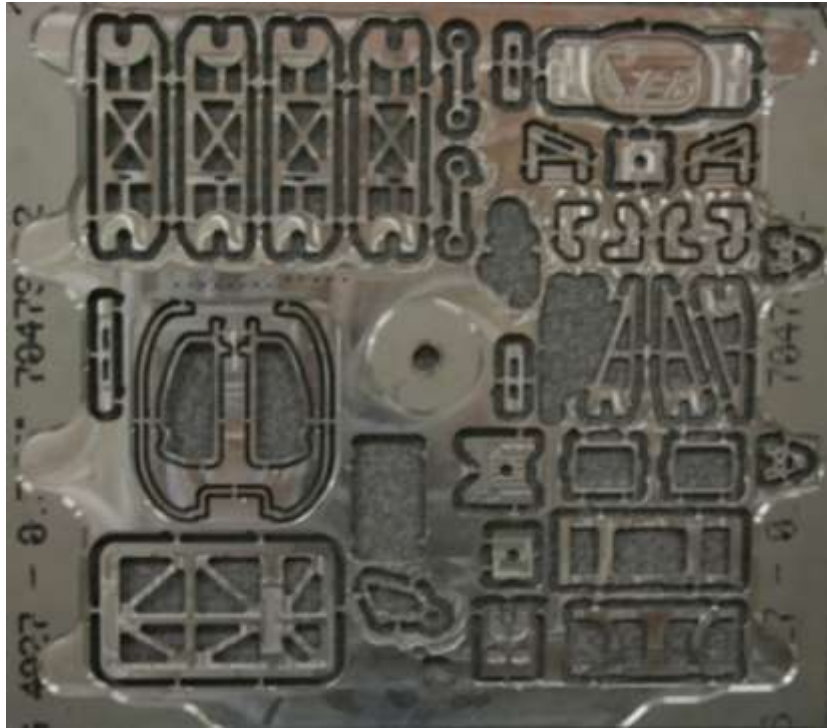
Figure 6.18 Aluminum alloy plate cut by CNC machining center
