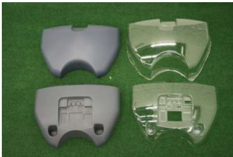
Figure 6.21 Vacuum Forming Machine, Model: Formech Midi (Top) Cover Molds and Plastic Covers (Bottom)
