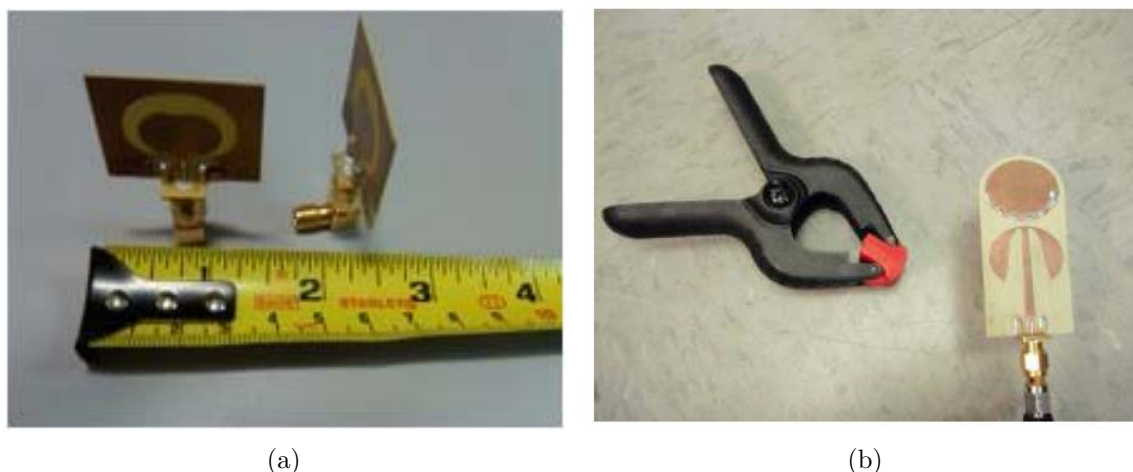
Figure 7.1: (a) UWB antennas manufactured by the Virginia Tech Antenna Group (VTAG). and (b) UWB antennas from Time Domain Corporation.
