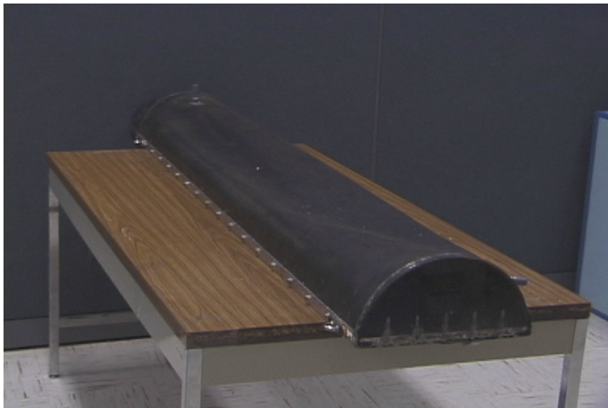
Figure 5.32: Side-view of the first hemi-cylindrical flexible composite breakwater model.
