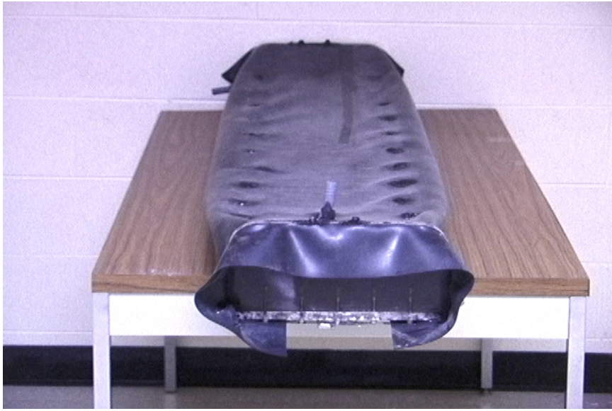
Figure 5.8: Front-view of the rectangular flexible breakwater model.
