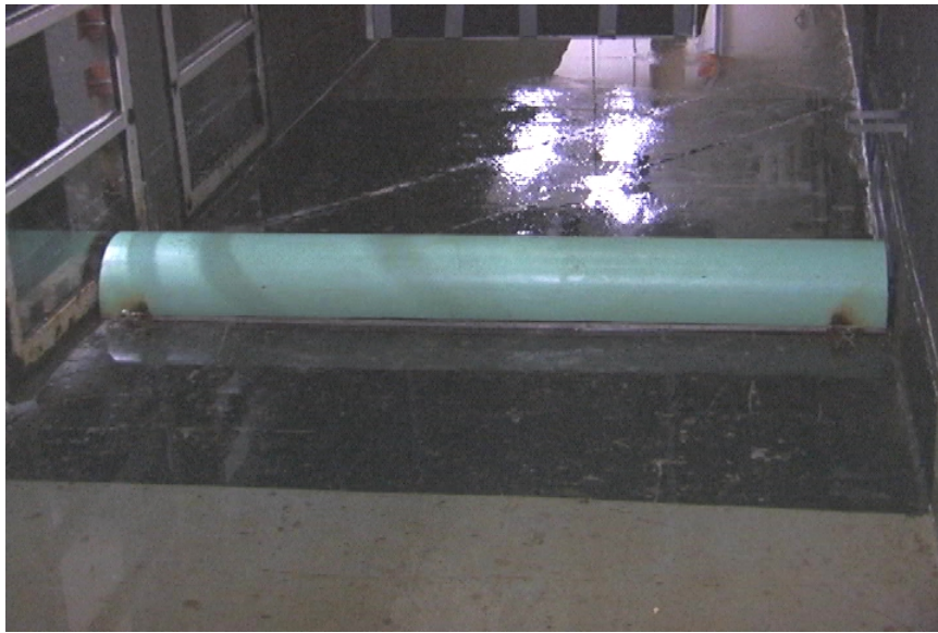
Figure 5.25: Hemi-cylindrical rigid breakwater model anchored rigidly at the wave tank floor.
