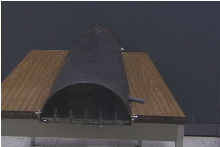
Figure 5.31: Front-view of the first hemi-cylindrical flexible composite breakwater model.
