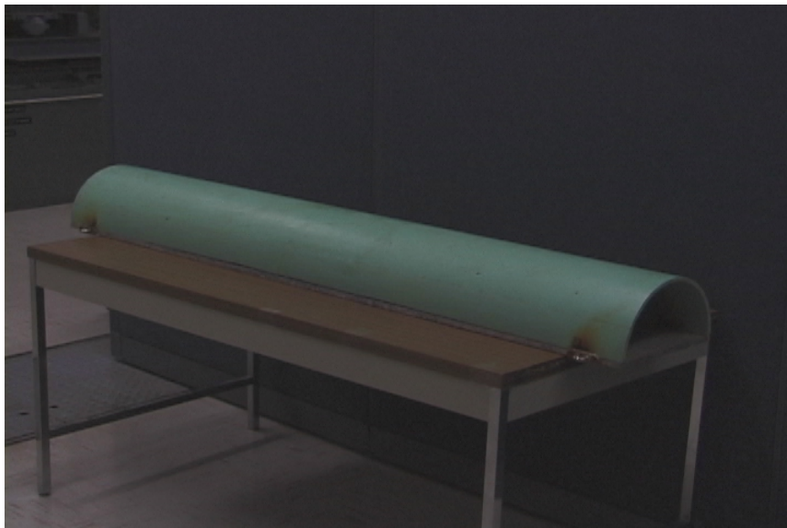
Figure 5.21: Side-view of hemi-cylindrical rigid breakwater model.
