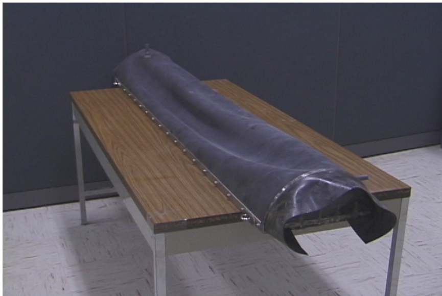
Figure 5.24: Side-view of hemi-cylindrical flexible breakwater model.
