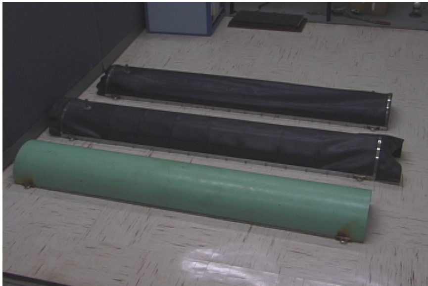
Figure 2.8: Side-view of hemi-cylindrical, rigid, second and first flexible composite breakwater models.
