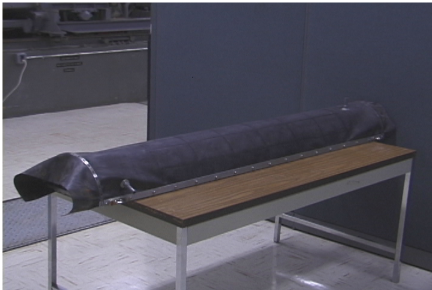
Figure 5.39: Side-view of the second hemi-cylindrical flexible composite breakwater model.
