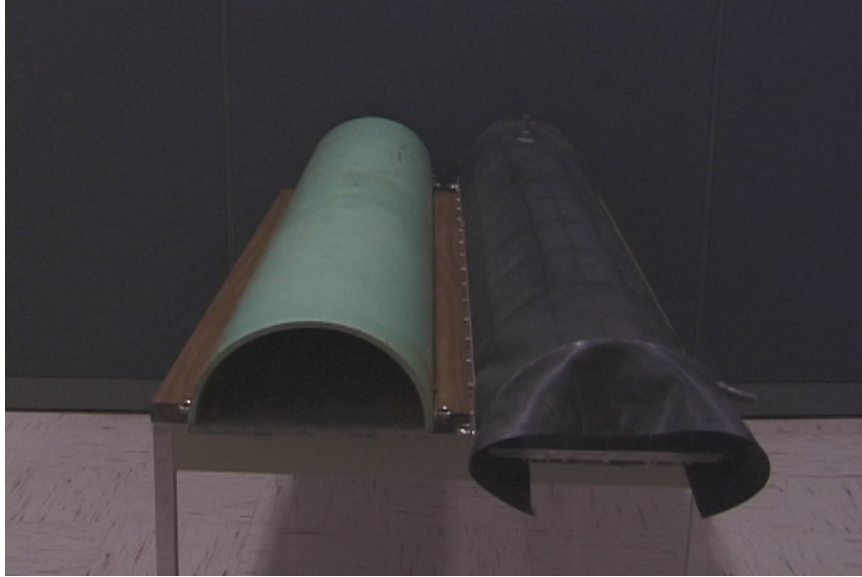
Figure 5.40: Front-view of the hemi-cylindrical rigid and second flexible composite breakwater models.
