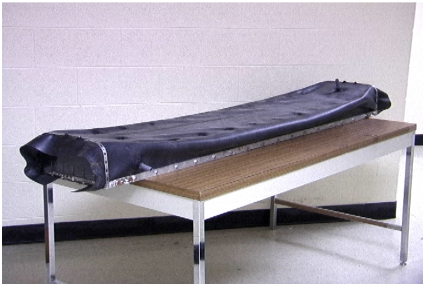
Figure 5.9: Side-view of the rectangular flexible breakwater model.
