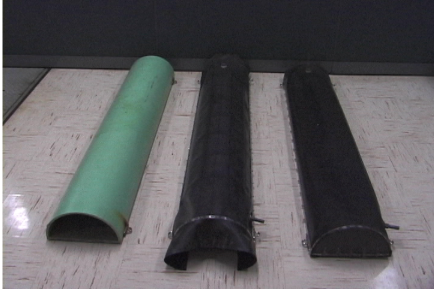
Figure 2.7: Front-view of hemi-cylindrical, rigid, second and first flexible composite breakwater models, seen from the left.
