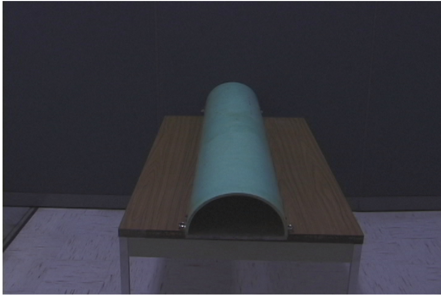
Figure 5.20: Front-view of hemi-cylindrical rigid breakwater model.
