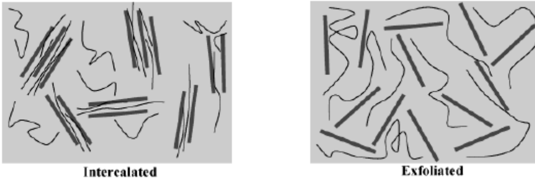
Figure 2.1: Schematic illustrations of two types of polymer-layered silicate morphologies: (left) intercalated and (right) exfoliated [2].
