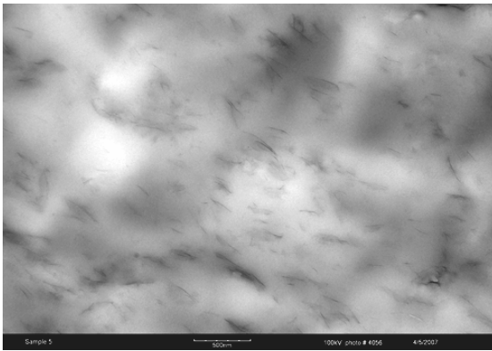
Figure 5.4: METH#3+MA: 4.2 wt% (Left = 17,000x, Right = 34,000x)
