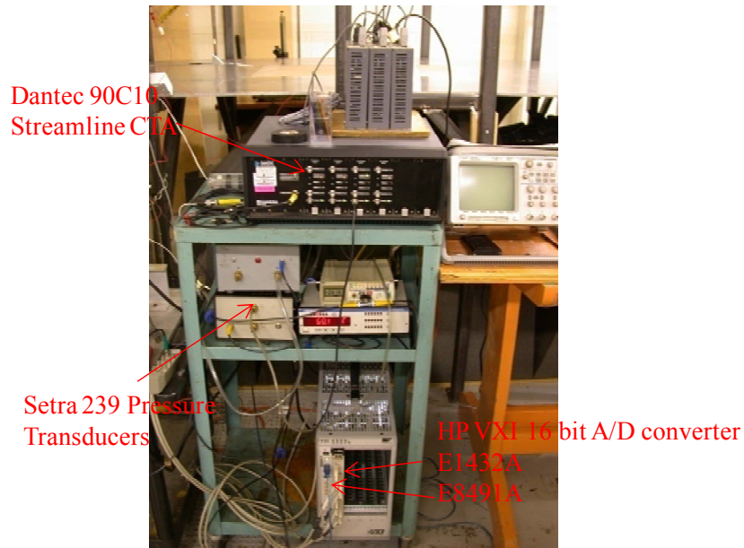
Figure 2.13 Single sensor hotwire measurement system setup
