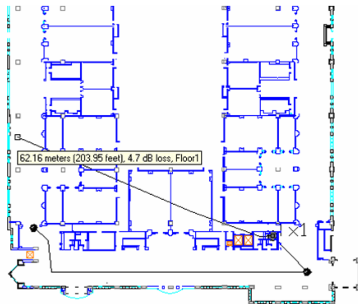
Figure 4.4: Screen capture from SitePlanner ® from Wireless Valley Communications, Inc. showing the placement of a coaxial cable within the site-specific model.
