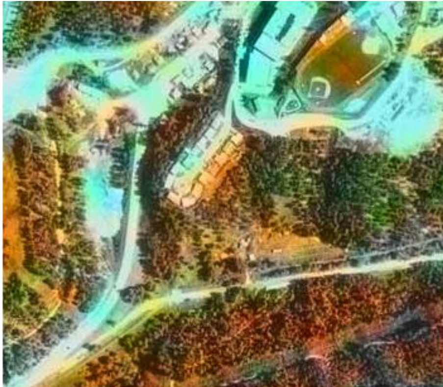
Figure 2.8: An example GeoTIFF file. The color of each pixel in the file corresponds to a specific range of elevation for the terrain shown at that pixel. [183]
