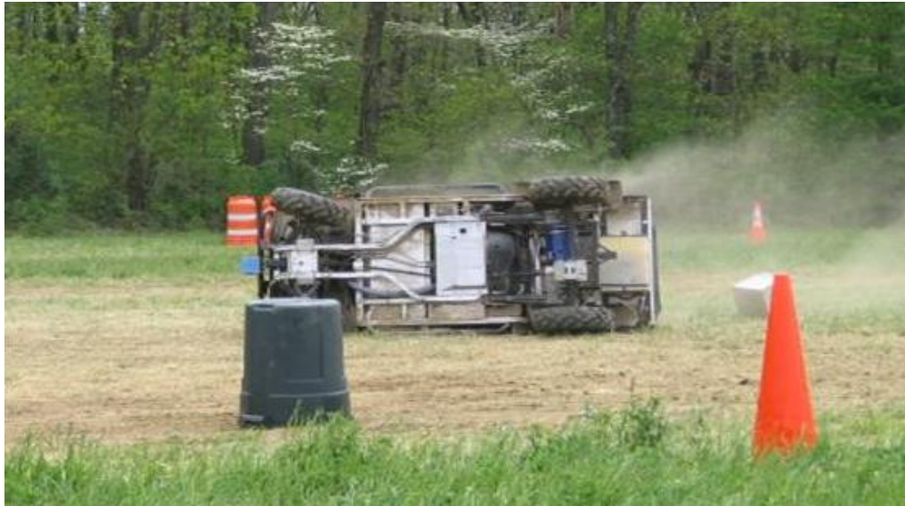
Figure 1.1: Virginia Tech’s Rocky rolls over as a result of attempting a dynamically infeasible maneuver. This rollover occurred during evaluation testing for the DARPA Grand Challenge
